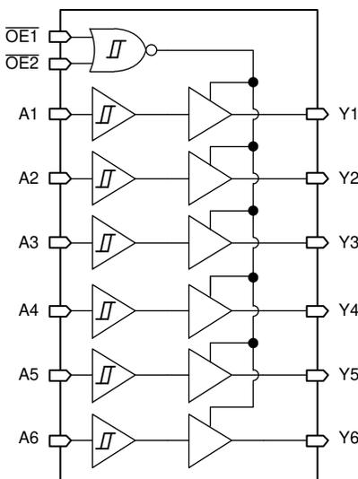
Figure 8-1. Logic Diagram (Positive Logic) for SN74HCS365-Q1
