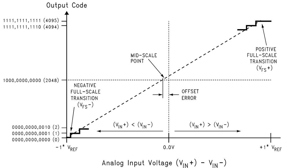
Figure 2. Transfer Characteristic
