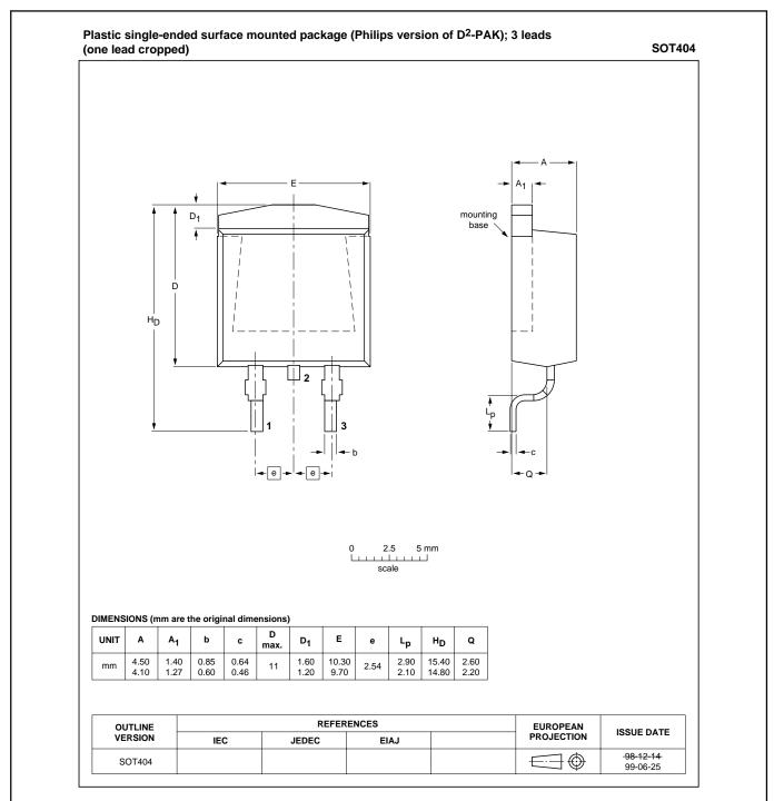
Fig.2. SOT404 surface mounting package<sup>1</sup>, centre pin connected to mounting base.
