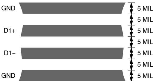
**Figure 17. Arrangement of Signal Tracks**
