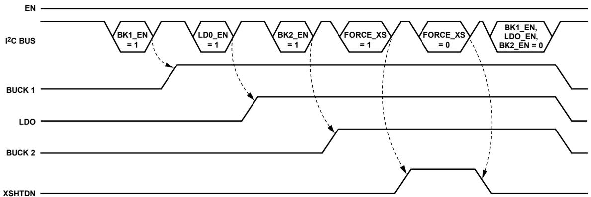
Figure 26. Individual Activation Through I<sup>2</sup>C Commands
