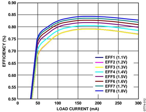
Figure 12. Buck 2 Efficiency vs. Load Current
