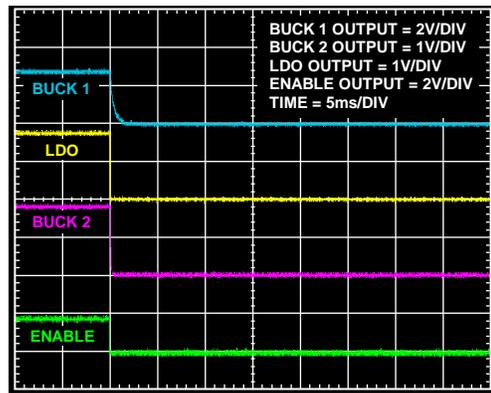
Figure 21. Three Regulators Turned Off by Sequencer
