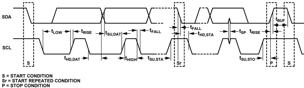
Figure 3. I<sup>2</sup>C Interface Timing Diagram
