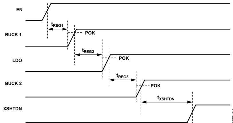
Figure 22. Automatic Sequencing with EN Low-to-High Transition
