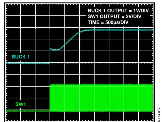
Figure 17. Buck 1 Enable Startup
