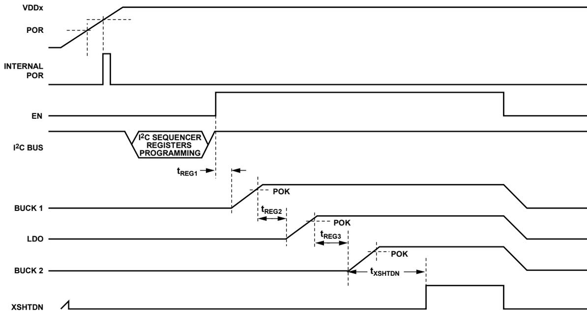
Figure 24. Activation Command Using the EN Pin
