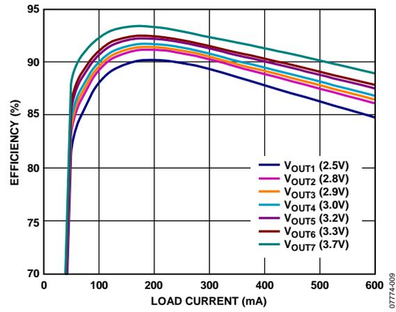
Figure 9. Buck 1, Efficiency vs. Load Current
