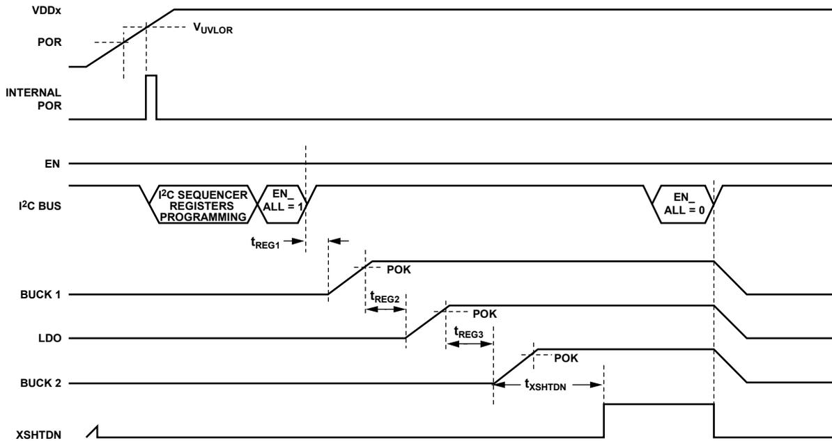
Figure 23. Regulators Are Activated by I<sup>2</sup>C Command
