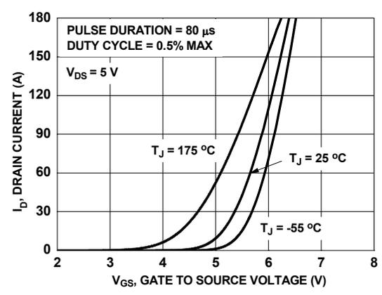
Figure 5. Transfer Characteristics
