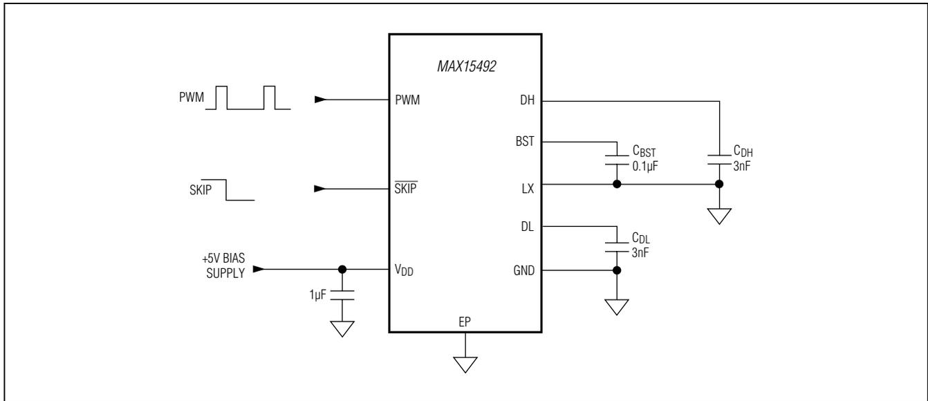
Figure 1. Test Circuit
