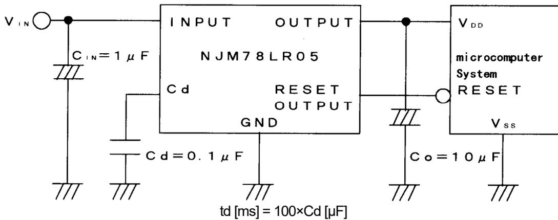
Note 1 : When the capacitance  $C_d$  is too large, the actual delay time is shorter than the calculated result because an electrical charge of  $C_d$  is discharged incompletely.
