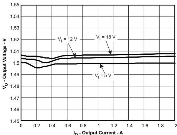
Figure 5. VO2=1.5V Output Voltage vs Output Current
