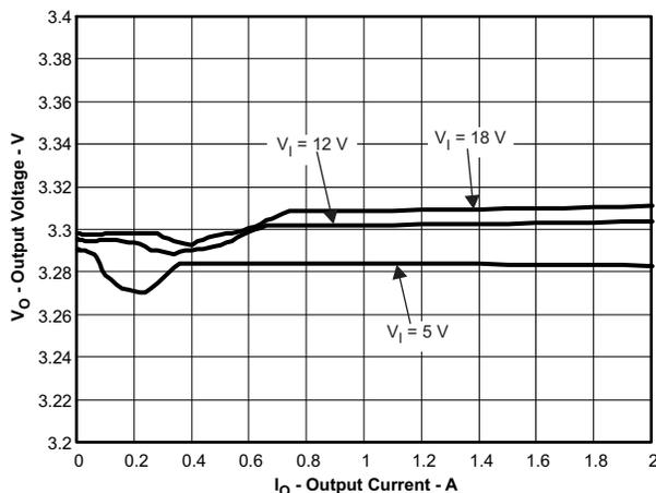
Figure 4. VO1=3.3V Output Voltage vs Output Current
