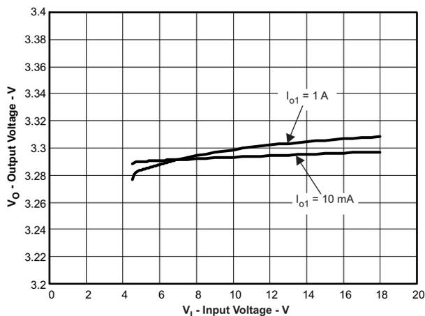
Figure 6. VO1=3.3V Output Voltage vs Input Voltage
