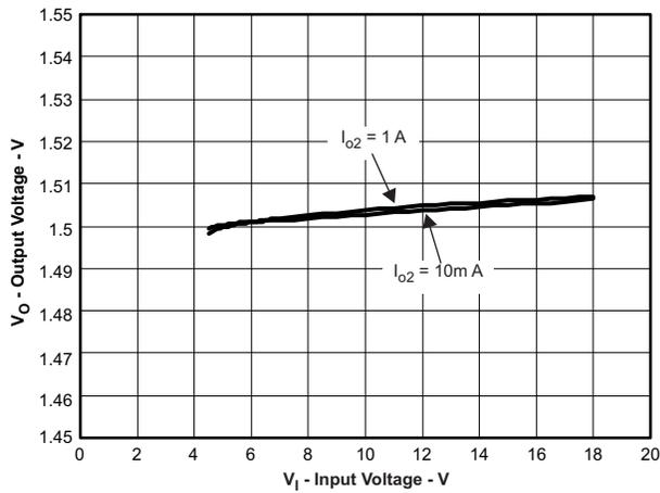
Figure 7. VO2=1.5V Output Voltage vs Input Voltage
