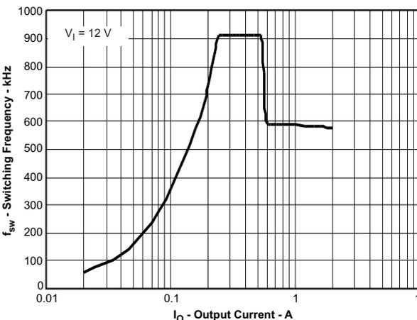
Figure 18.  $V_{O1}=3.3\text{V}$ , SW-frequency vs Output Current
