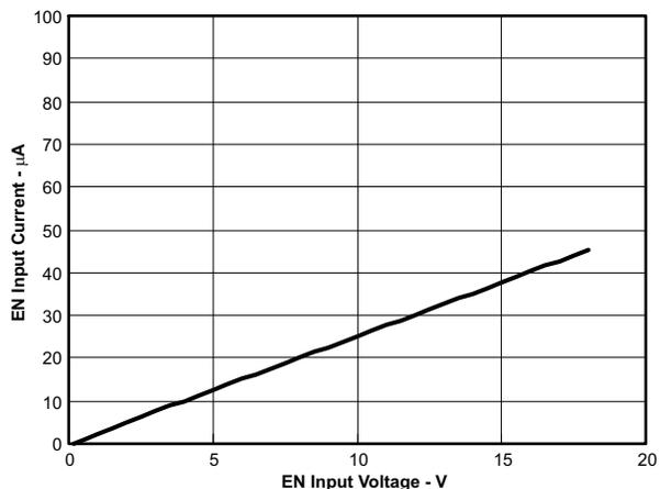
Figure 3. EN Current vs EN Voltage (VEN=12V)
