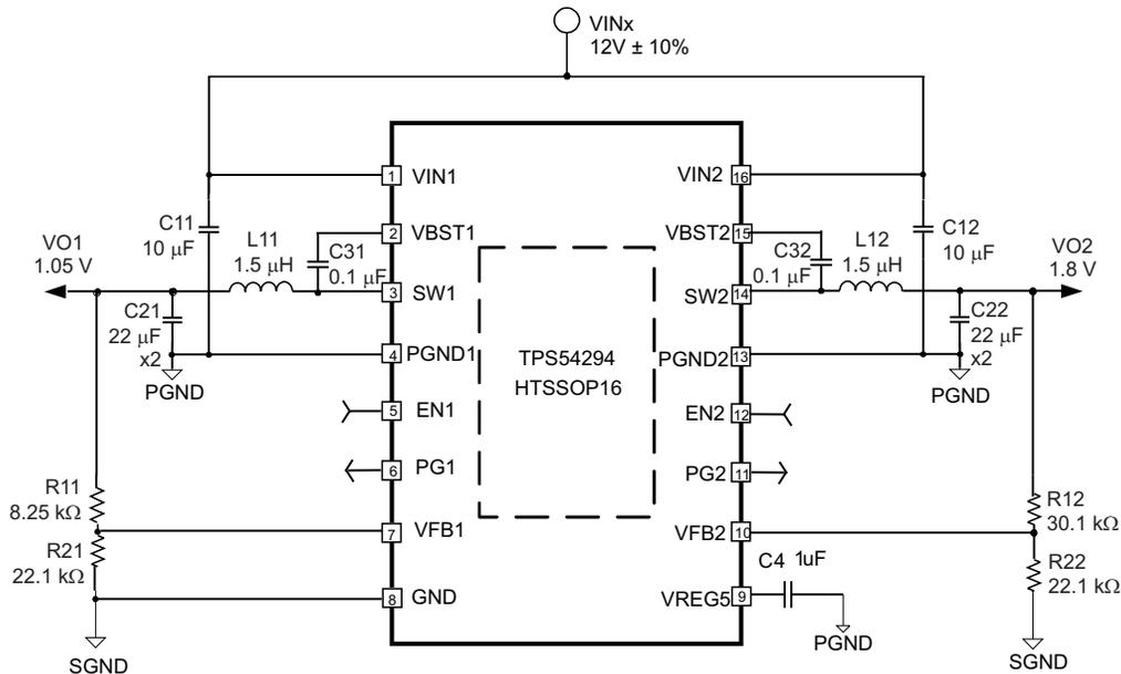
Figure 24. Schematic Diagram for the Design Example
