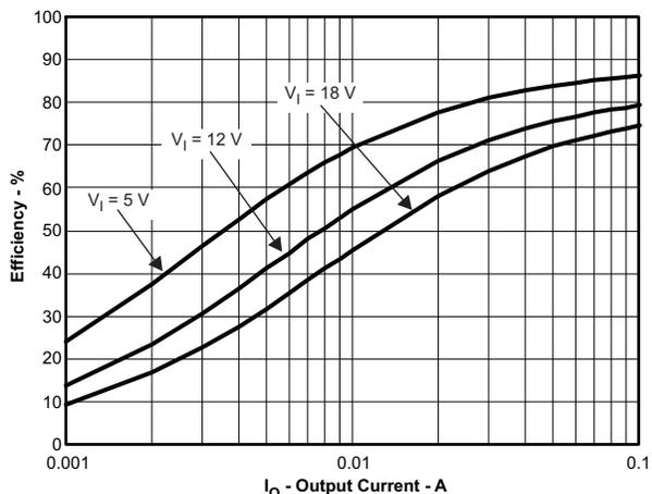
Figure 15.  $V_{O2}=1.5\text{V}$ , Efficiency vs Output Current
