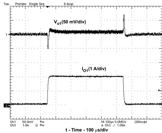
Figure 8. VO1=3.3V, 0A to 2A Load Transient Response
