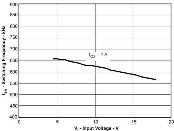
Figure 17.  $V_{O2}=1.5\text{V}$ , SW-frequency vs Input Voltage
