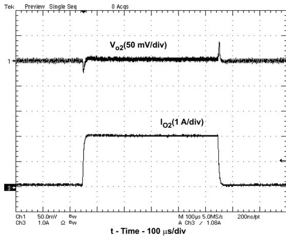
Figure 9. VO2=1.5V, 0A to 2A Load Transient Response
