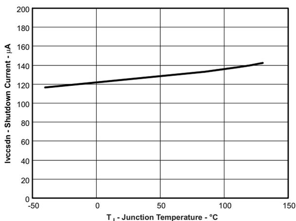
Figure 2. Input Shutdown Current vs Junction Temperature
