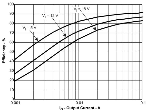
Figure 13.  $V_{O1}=3.3\text{V}$ , Efficiency vs Output Current
