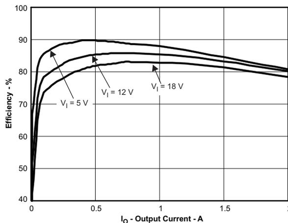
Figure 14.  $V_{O1}=1.5\text{V}$ , Efficiency vs Output Current
