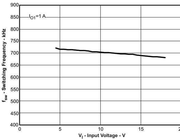
Figure 16.  $V_{O1}=3.3\text{V}$ , SW-frequency vs Input Voltage
