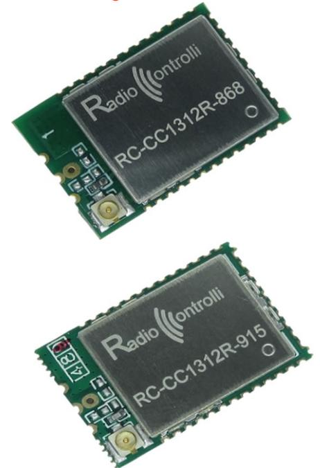
The **RC-CC1312R-XXX** module is based on Texas Instruments CC1312R1F3RGZ component. This device combines a flexible, very low power RF transceiver with a powerful 48 MHz ARM Cortex M4F CPU in a platform supporting multiple physical layers and RF standard. This device is pin to pi compatible with the module RC-CC1310-XXX.
