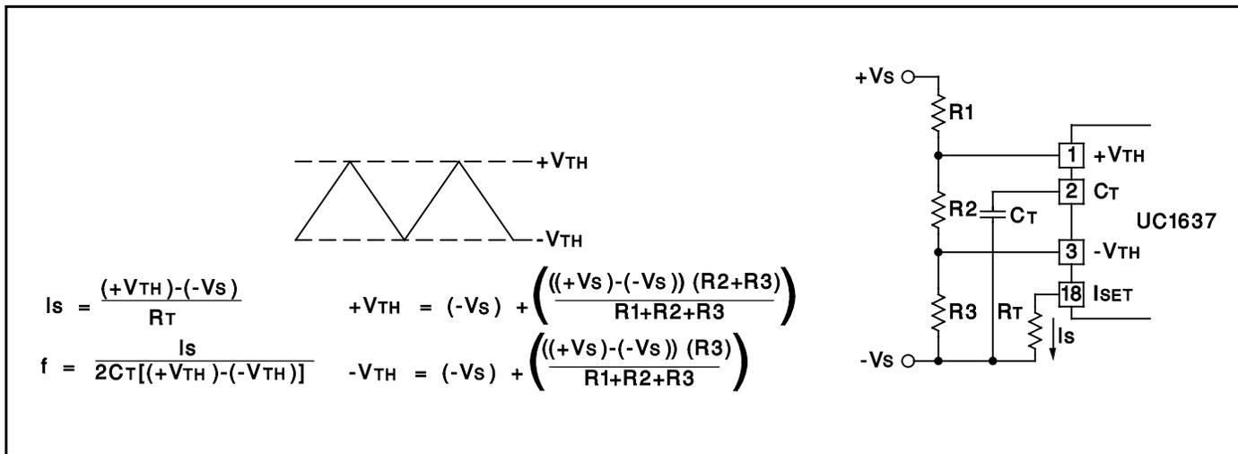
Figure 1. Oscillator Setup
