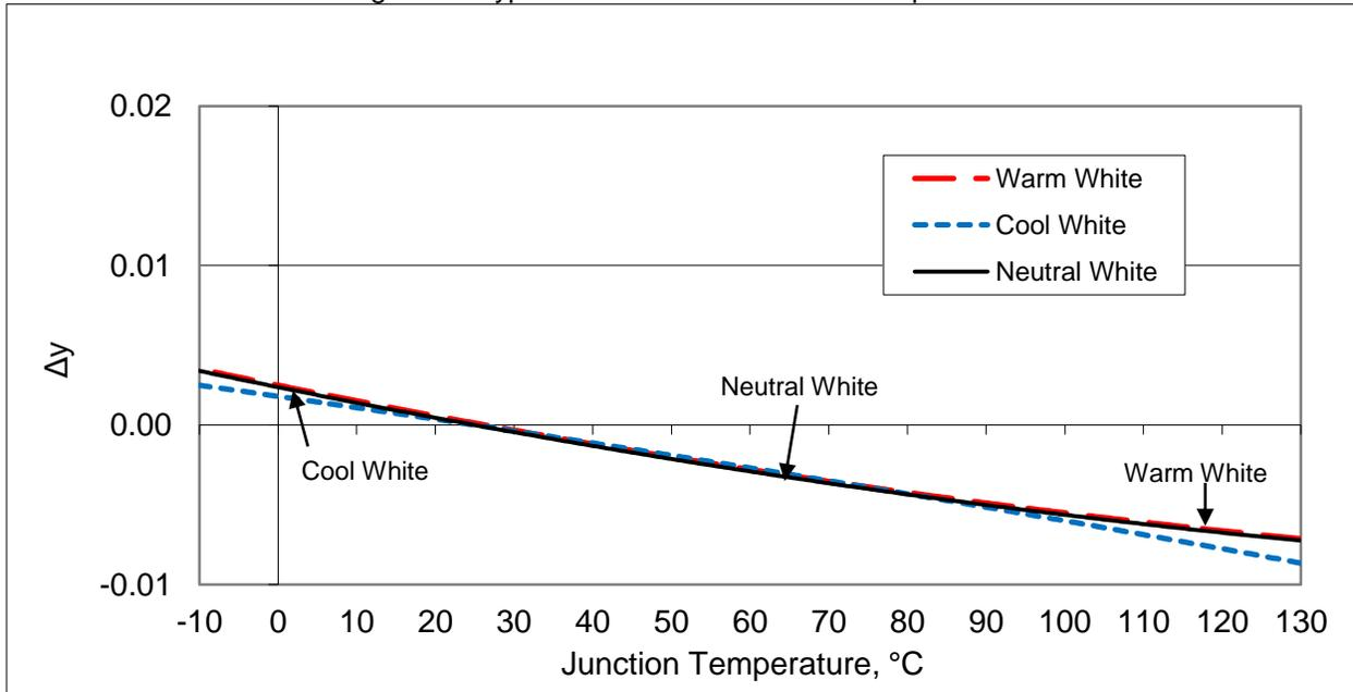
Figure 5: Typical ccy Shift vs. Junction Temperature
