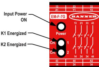
The Safety Extension Module offers an output circuit at terminals Y1 and Y2 which provides K1 and K2 contact status information for connection to the monitoring input of the Primary Safety Device (see [Figure 1](#) on page 5). This monitoring circuit prevents the Primary Safety Device from being reset if contacts of either K1 or K2 of the Extension Module fail in a shorted condition.
