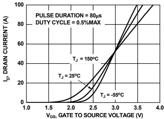
Figure 5. Transfer Characteristics
