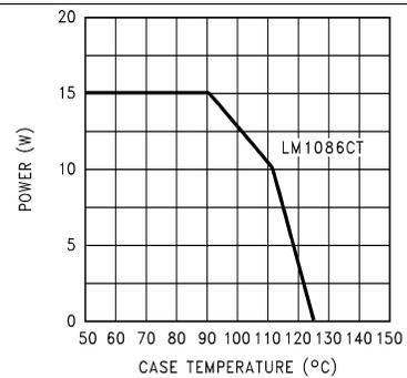
Figure 6. Maximum Power Dissipation vs Temperature
