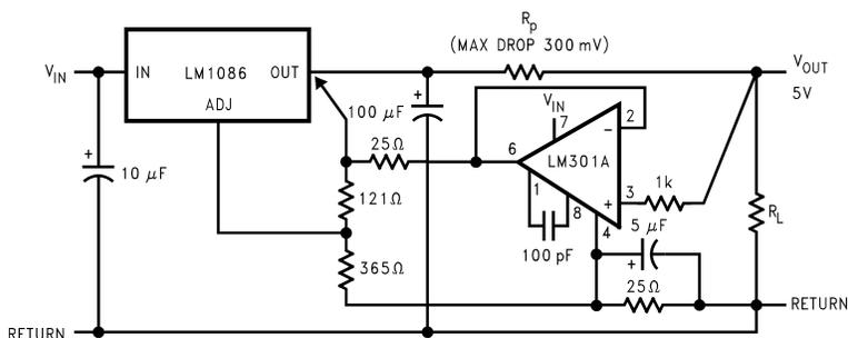
Figure 28. Remote Sensing
