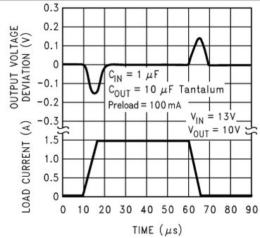
Figure 12. Load Transient Response
