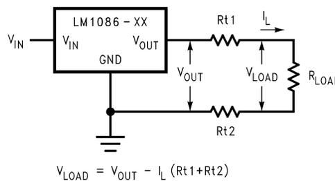
**Figure 14. Typical Application Using Fixed Output Regulator**
