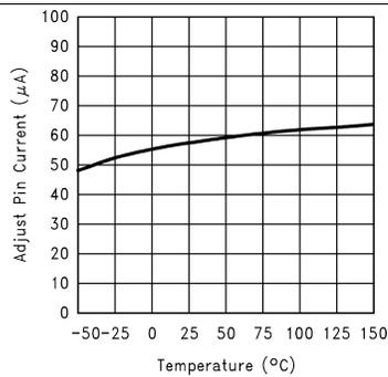
Figure 5. Adjust Pin Current vs Temperature
