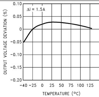
Figure 3. Load Regulation vs Temperature
