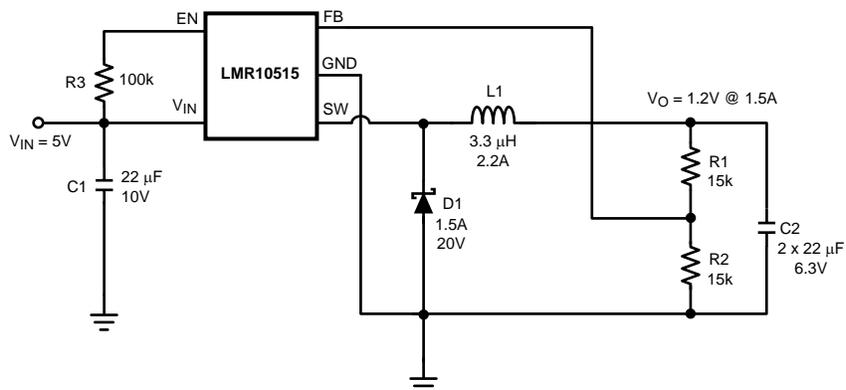
Figure 21. Lmr10515x (1.6mhz): Vin = 5v, Vo = 1.2v @ 1.5a
