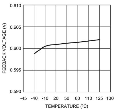
Figure 11.  $V_{FB}$  vs Temperature
