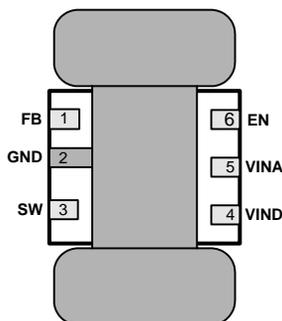
Figure 26. 6-Lead WSON PCB Dog Bone Layout
