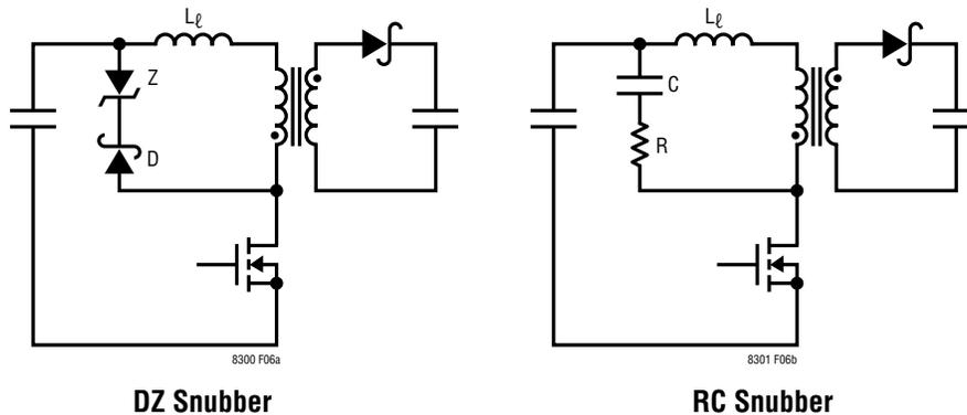
Figure 6. Snubber Circuits
