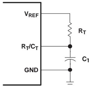
Figure 3. Oscillator Section
