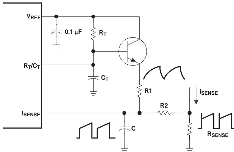
Figure 6. Slope Compensation
