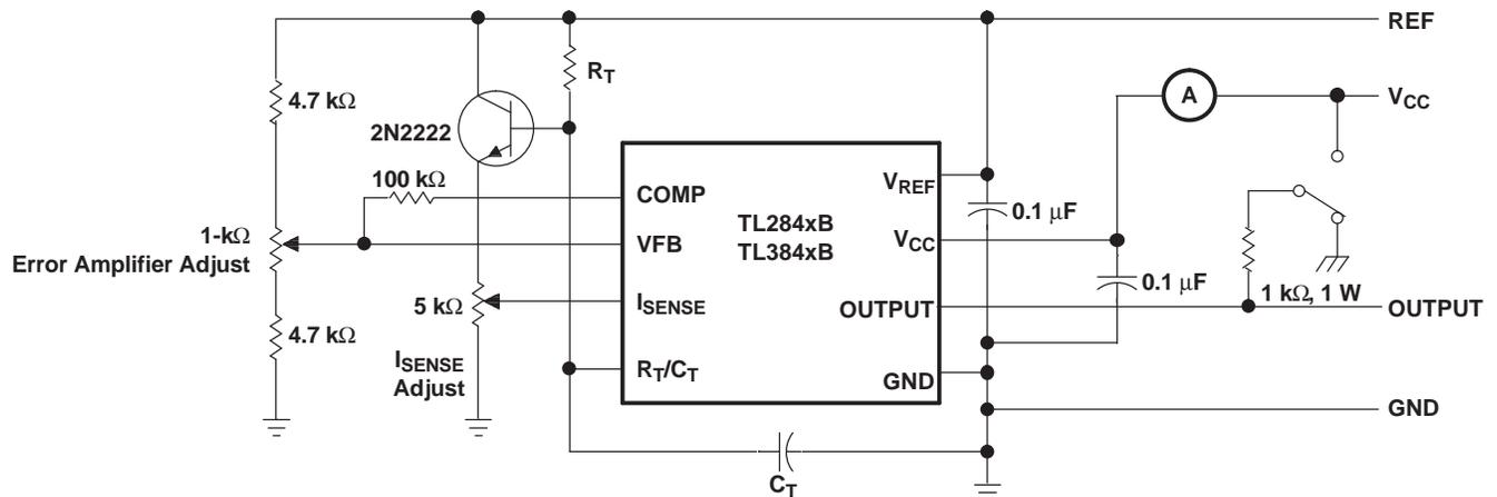
Figure 4. Open-Loop Laboratory Test Fixture
