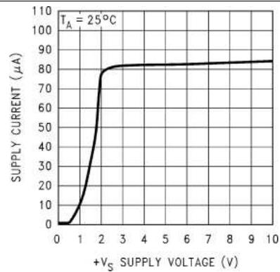
**Figure 10. Supply Voltage vs Supply Current**
