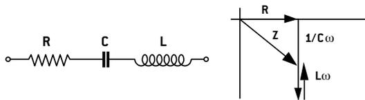
**R:** equivalent series resistance of the capacitor (leads, contacts, MnO<sub>2</sub>, dielectric losses)
