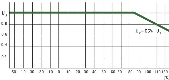
For the types which can be used up to  $200^{\circ}\text{C}$ , the voltage must be derated between  $+85^{\circ}\text{C}$  and  $+200^{\circ}\text{C}$  according to the following curve.
