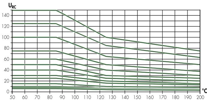
The **category voltage ( $U_C$ )** is consequently the maximum DC voltage which can be applied continuously at  $+125^{\circ}\text{C}$ .
