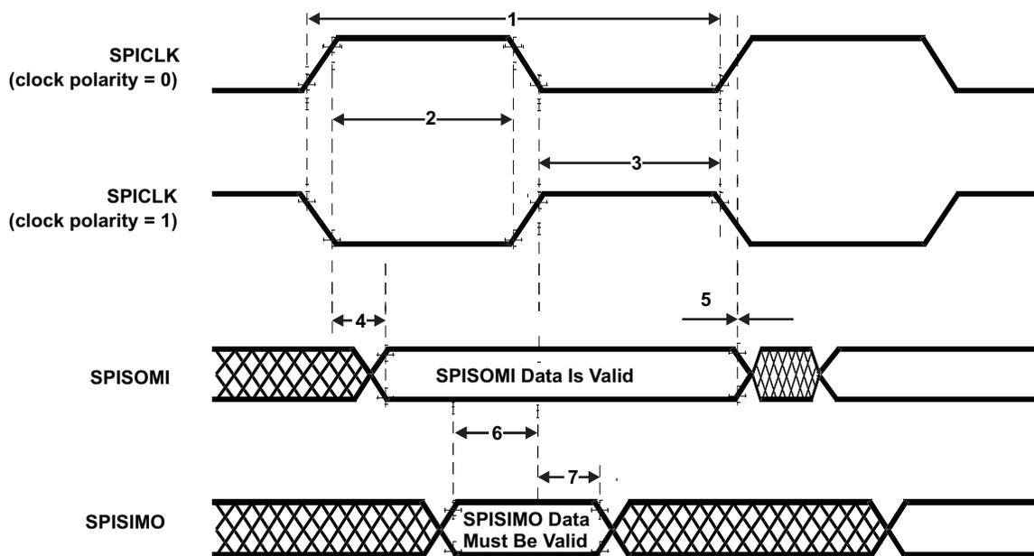
Figure 7-10. SPI Slave Mode External Timing (CLOCK PHASE = 0)
