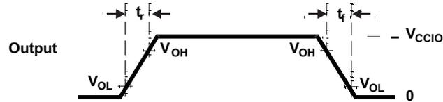
Figure 5-3. CMOS-Level Outputs
