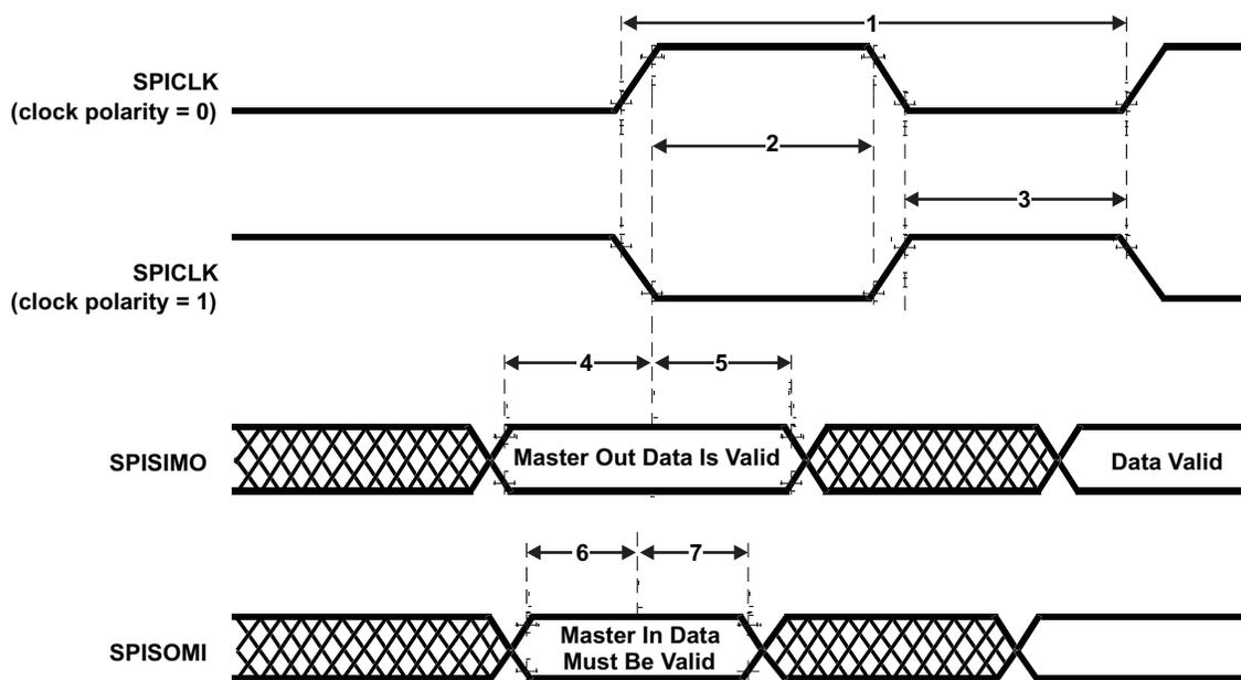
Figure 7-8. SPI Master Mode External Timing (CLOCK PHASE = 1)
