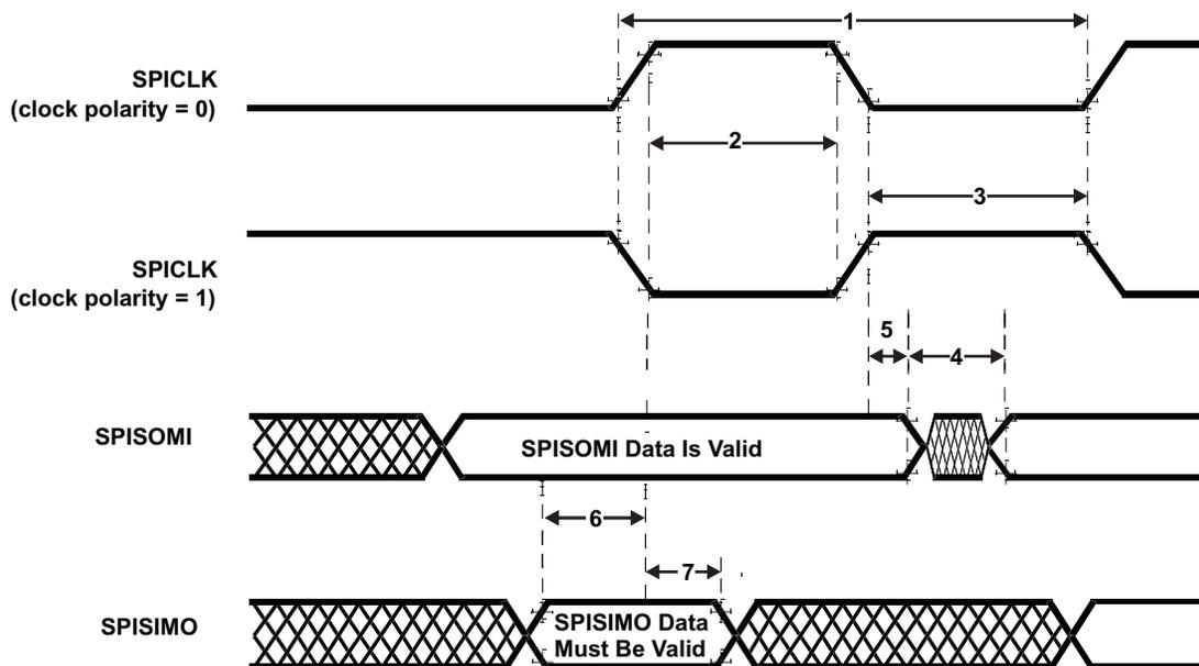
Figure 7-12. SPI Slave Mode External Timing (CLOCK PHASE = 1)
