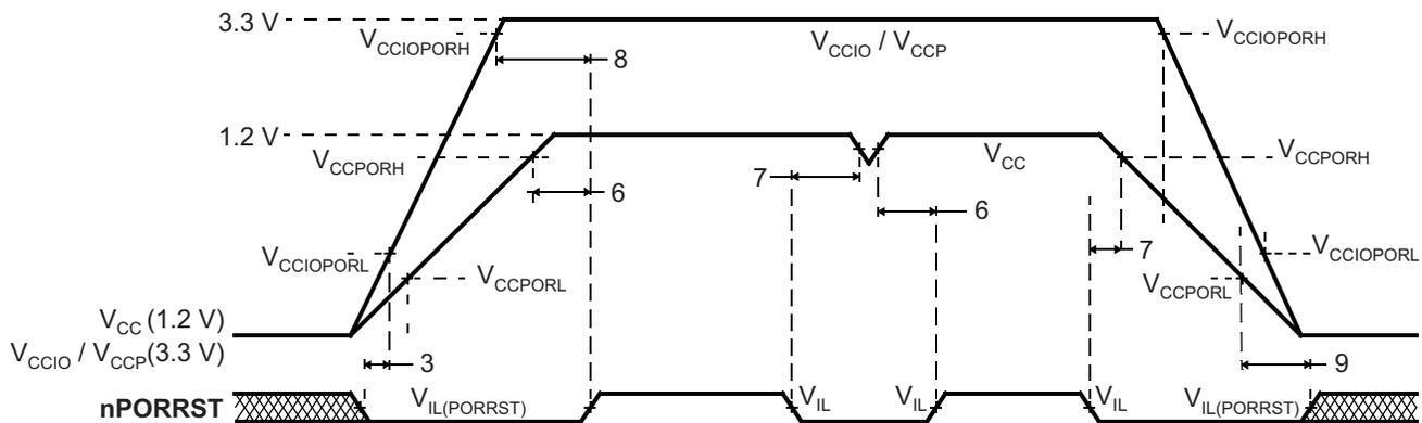
Note: There is no timing dependency between the ramp of the  $V_{CCIO}$  and the  $V_{CC}$  supply voltage; this is just an example.
