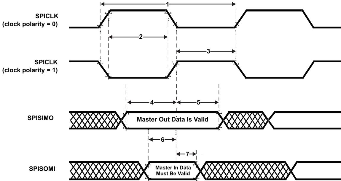
Figure 7-6. SPI Master Mode External Timing (CLOCK PHASE = 0)
