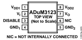
Figure 3. Pin Configuration
