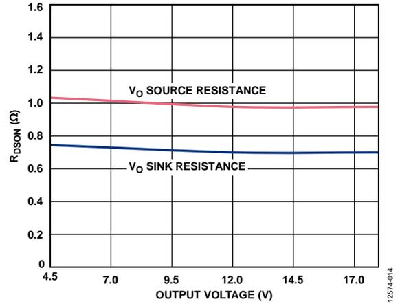
Figure 14. Typical Output Resistance ( $R_{DS(on)}$ ) vs. Output Voltage
