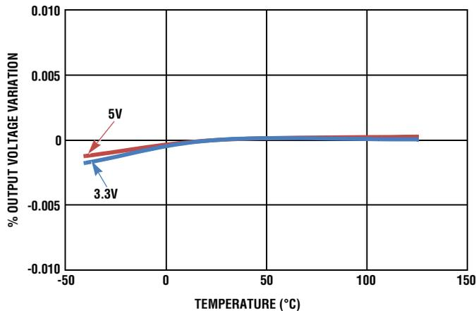
FIGURE 6. OUTPUT VOLTAGE vs TEMPERATURE (LOAD = 50mA)
