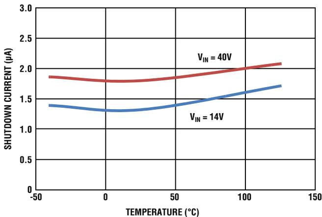
FIGURE 5. SHUTDOWN CURRENT vs TEMPERATURE (EN = 0)
