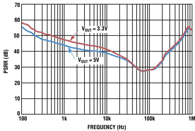
FIGURE 9. POWER SUPPLY REJECTION RATIO (LOAD = 50mA)
