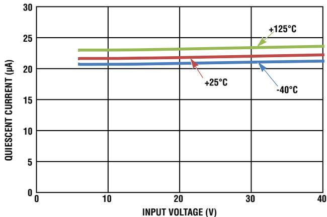
FIGURE 4. QUIESCENT CURRENT vs INPUT VOLTAGE (NO LOAD)
