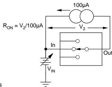
ON RESISTANCE vs ANALOG INPUT VOLTAGE
