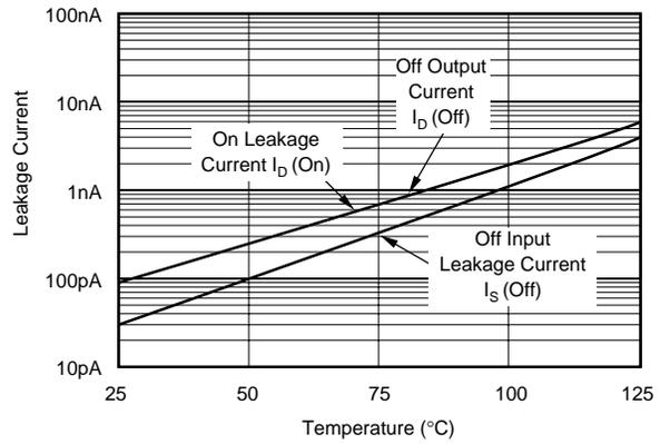
NOTE: (1) Two measurements per channel: +10V/-10V and -10V/+10V. (Two measurements per device for  $I_D$ (Off): +10V/-10V and -10V/+10V).
