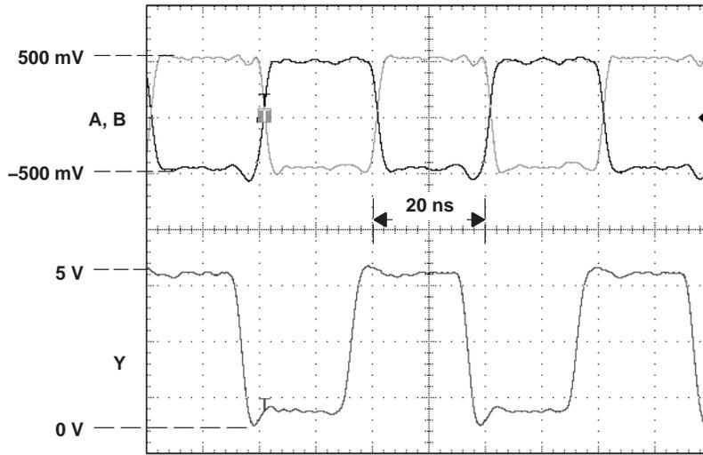
Figure 10. Receiver Inputs and Outputs, 50 Mbps Signaling Rate
