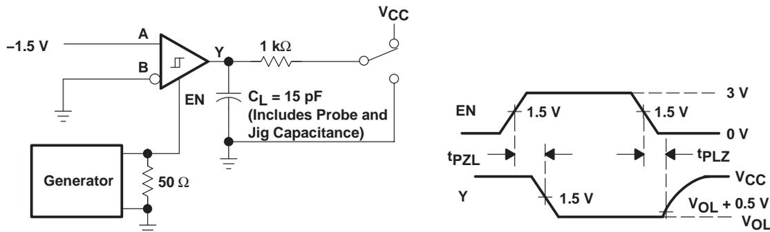
Figure 4. Test Circuit Waveforms,  $t_{pZL}$  and  $t_{pLZ}$
