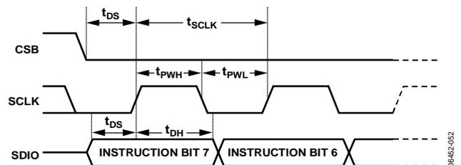
Figure 55. Timing Diagram for 3-Wire Interface Register Write
