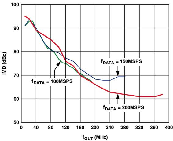
Figure 20. AD9779A Third-Order IMD vs.  $f_{OUT}$ , 4x Interpolation
