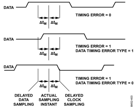
Figure 87. Timing Diagram of Margin Test Data
