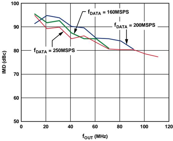
Figure 18. AD9779A Third-Order IMD vs.  $f_{OUT}$ , 1x Interpolation
