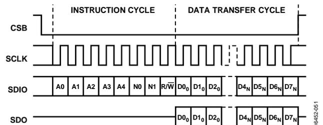
Figure 54. Serial Register Interface Timing, LSB First
