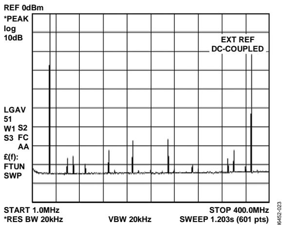
Figure 26. AD9779A Single Tone, 4x Interpolation,  $f_{DATA} = 100$  MSPS,  $f_{OUT} = 30$  MHz
