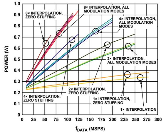
Figure 95. Total Power Dissipation, Dual DAC Mode
