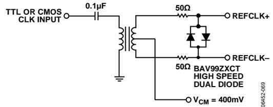
Figure 74. TTL or CMOS REFCLK Drive Circuit
