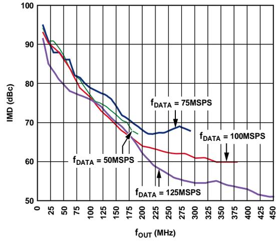
Figure 21. AD9779A Third-Order IMD vs.  $f_{OUT}$ , 8x Interpolation
