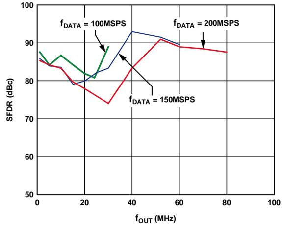
Figure 10. AD9779A In-Band SFDR vs.  $f_{OUT}$ , 4x Interpolation
