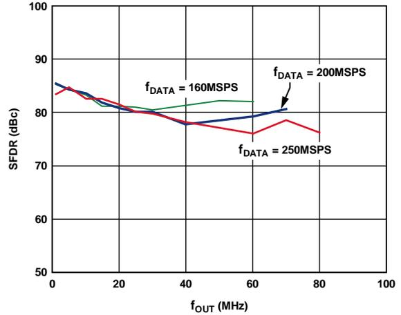
Figure 39. AD9778A In-Band SFDR vs.  $f_{OUT}$ , 2x Interpolation
