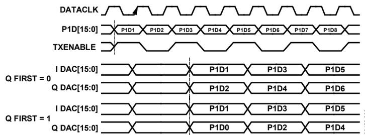
Figure 83. Single Port Mode Digital Interface Timing
