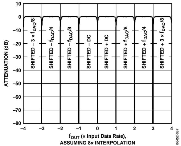
Figure 70. Shifted Bandwidths Accessible with the Filter Architecture
