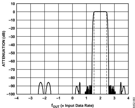
Figure 66. Interpolation/Modulation Combination of  $2f_{DAC}/8$  Filter
