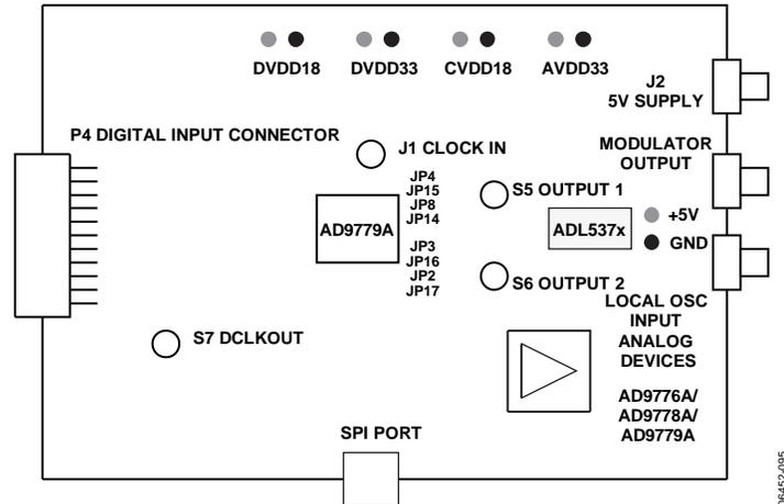
Figure 101. AD9776A/AD9778A/AD9779A Evaluation Board Showing All Connections
