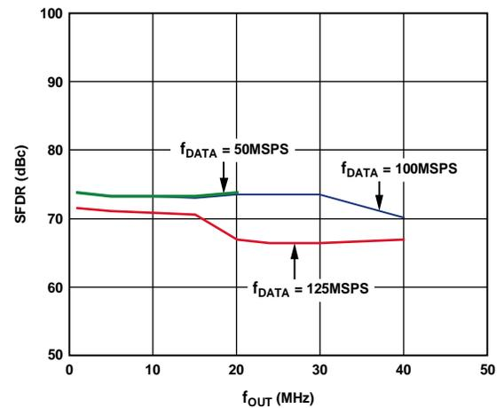
Figure 14. AD9779A Out-of-Band SFDR vs.  $f_{OUT}$ , 8x Interpolation
