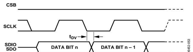
Figure 56. Timing Diagram for 3-Wire Interface Register Read
