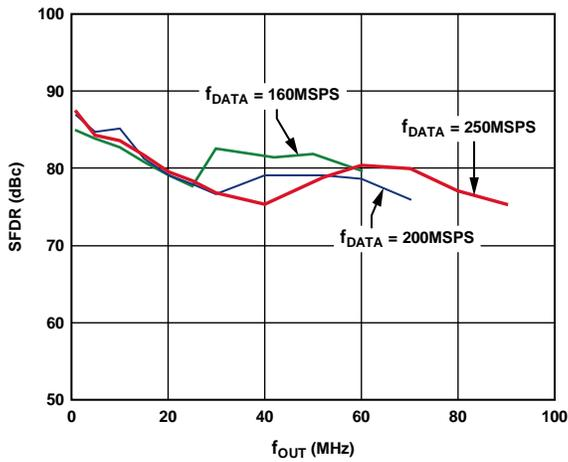
Figure 8. AD9779A In-Band SFDR vs.  $f_{OUT}$ , 1x Interpolation
