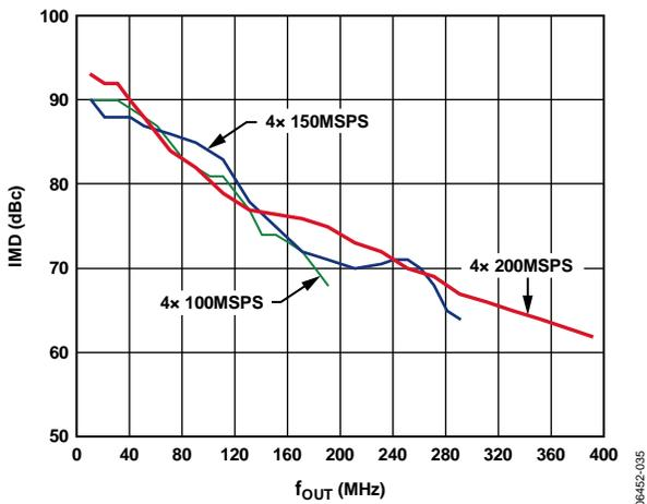
Figure 38. AD9778A IMD vs.  $f_{OUT}$ , 4x Interpolation
