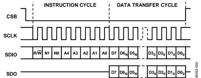
Figure 53. Serial Register Interface Timing, MSB First
