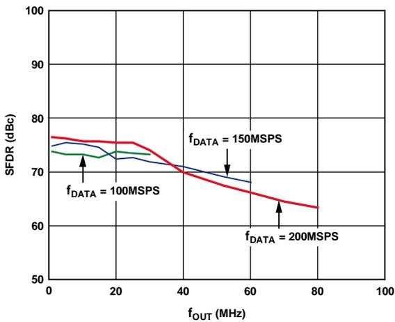
Figure 13. AD9779A Out-of-Band SFDR vs.  $f_{OUT}$ , 4x Interpolation
