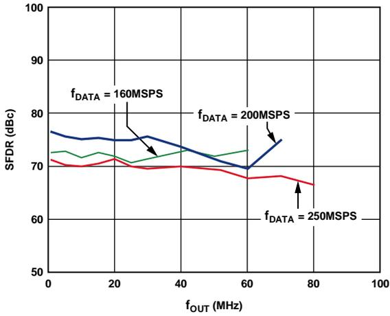
Figure 12. AD9779A Out-of-Band SFDR vs.  $f_{OUT}$ , 2x Interpolation
