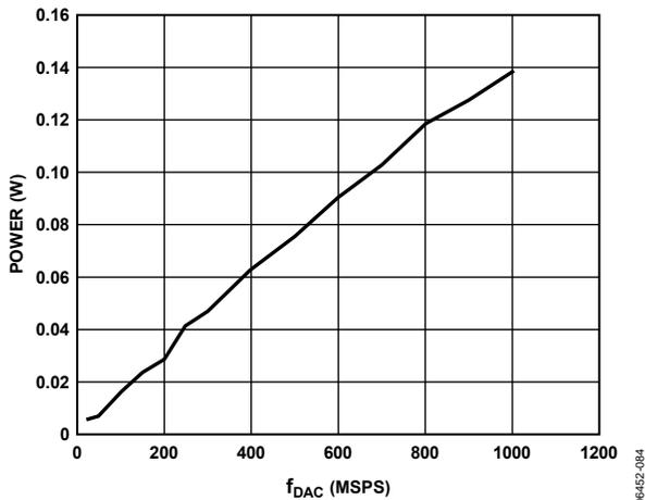
Figure 99. DVDD18 Power Dissipation of Inverse Sinc Filter
