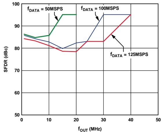
Figure 11. AD9779A In-Band SFDR vs.  $f_{OUT}$ , 8x Interpolation
