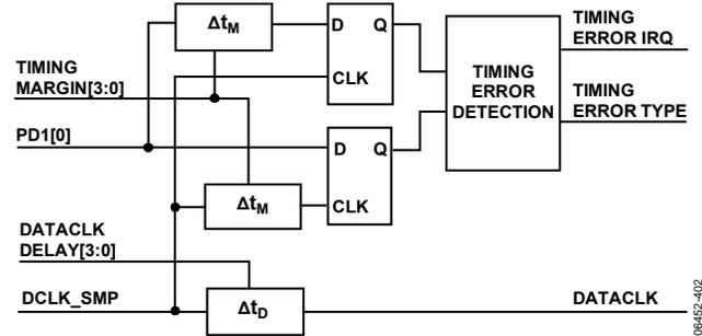
Figure 86. Timing Error Detection and Optimization Circuitry
