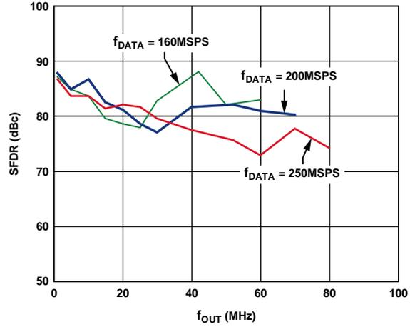
Figure 9. AD9779A In-Band SFDR vs.  $f_{OUT}$ , 2x Interpolation
