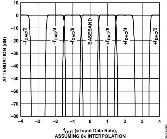
Figure 68. Traditional Bandwidth Options for TxDAC Output IF
