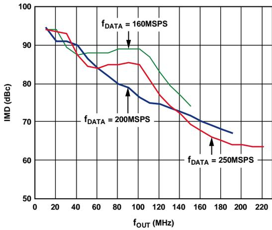
Figure 19. AD9779A Third-Order IMD vs.  $f_{OUT}$ , 2x Interpolation
