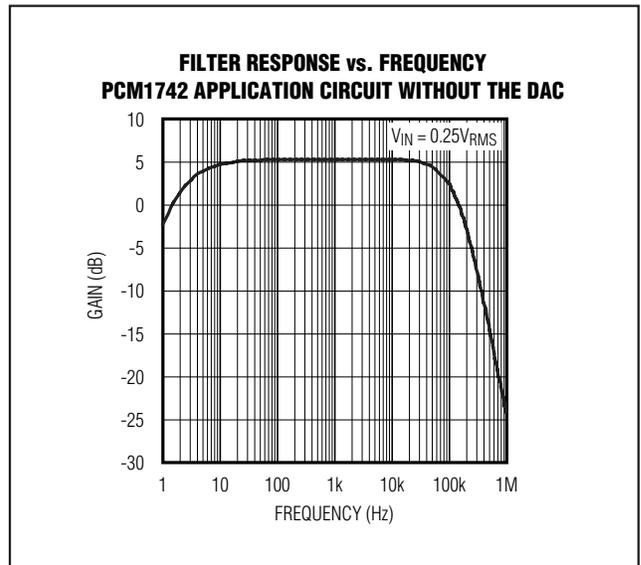
Figure 14. Filter Response of PCM1742 Filter Configuration
