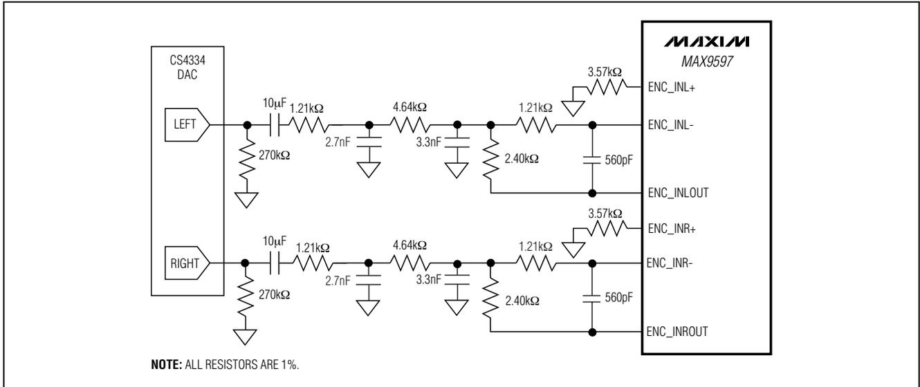
Figure 15. Lowpass Filter Configuration for the Cirrus CS4334
