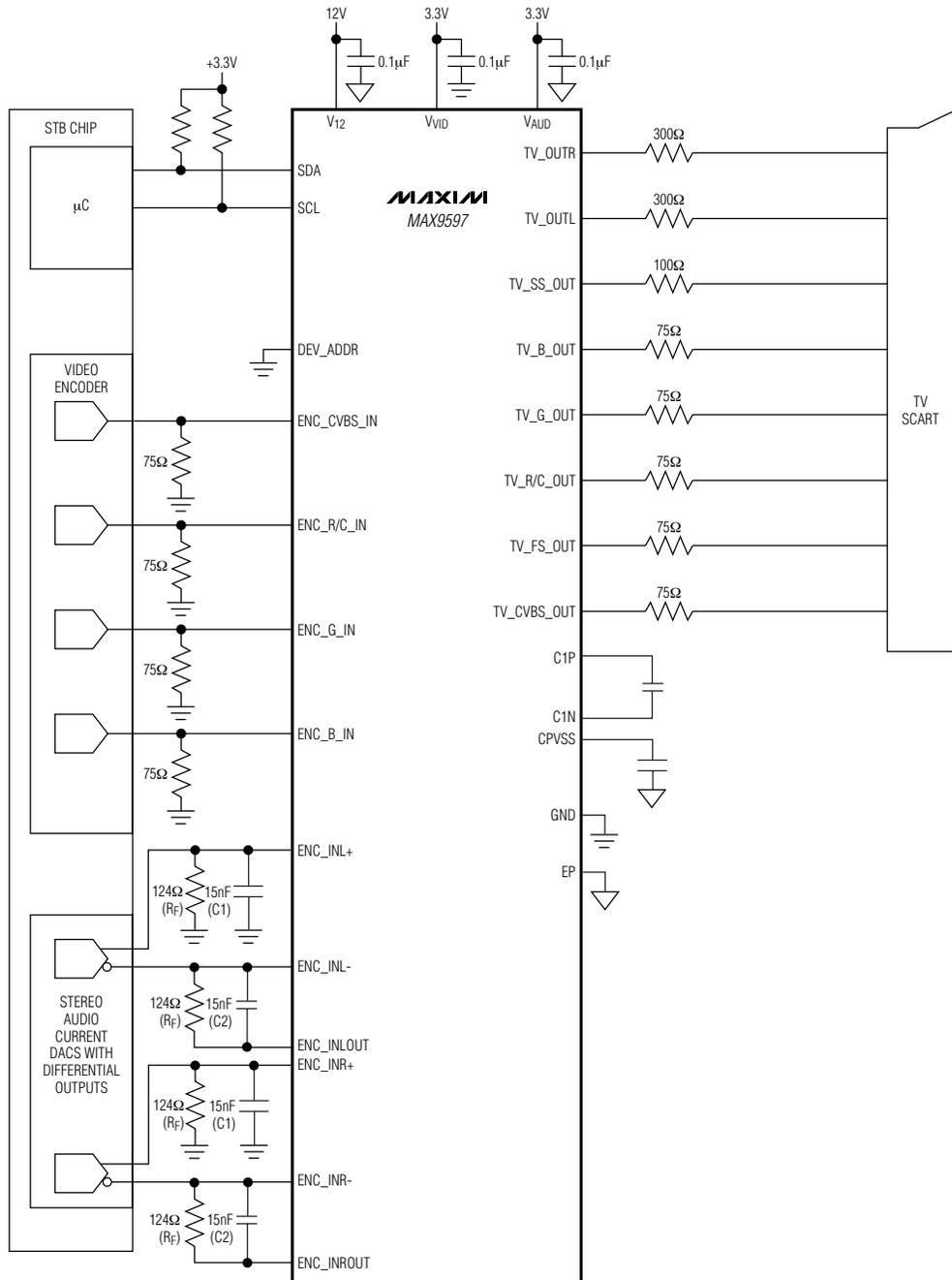
**NOTE:** OPTIONAL RESISTOR CAN BE PLACED FROM AUDIO DAC OUTPUTS TO GROUND TO DECREASE SWING AT AUDIO DAC OUTPUTS.
