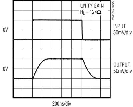
**INPUT-AMPLIFIER LARGE-SIGNAL TRANSIENT RESPONSE**
