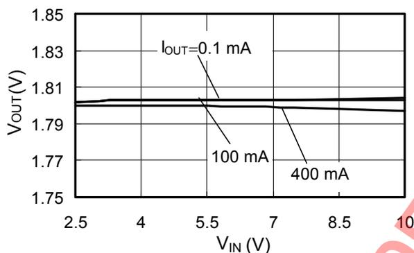
(11)  $V_{OUT} - V_{IN}$  3.3 V PWM/PFM 600 kHz
