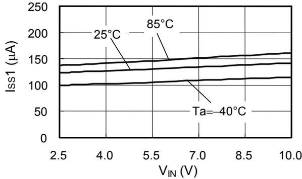
(2)  $I_{SS1} - V_{IN}$  S-8540/8541(600 kHz)
