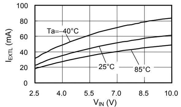
(7)  $V_{SH} - V_{IN}$  S-8540/8541
