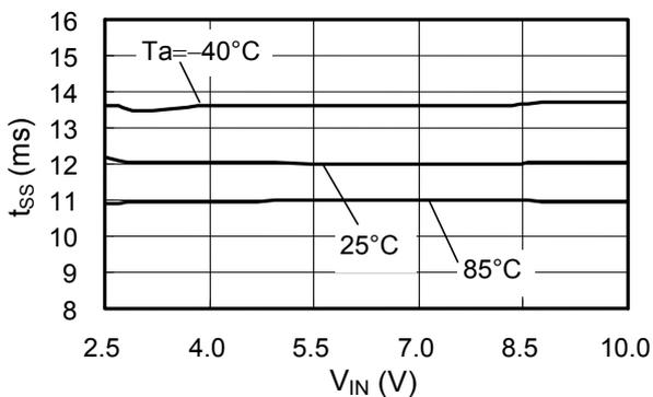
(10)  $V_{OUT} - V_{IN}$  1.8 V PWM/PFM 600 kHz
