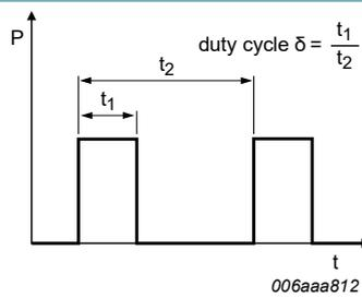
Fig. 17. Duty cycle definition
