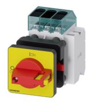
Load disconnector 3LD3, lu 25 A Main switch 3-pole Rated operating capacity at AC-23 A at 400V 9.0kW Front plate mounting Basic switch with Central hole mounting 22.5mm Toggle drive red / yellow 48x48 mm with auxiliary switch 1OE + 1S
