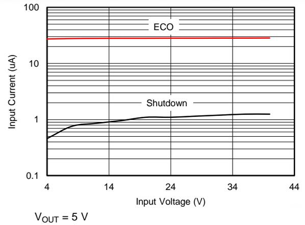
**Figure 4. Supply Current vs Input Voltage (No Load)**
