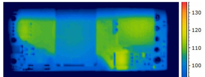
Figure 6. Thermal Image of CPE6B18 (6A output, 70C Ambient, 200lfm airflow, Vin = 24V, airflow from pin 3 to pin 1,  $T_{max} = 116^{\circ}C$ )
