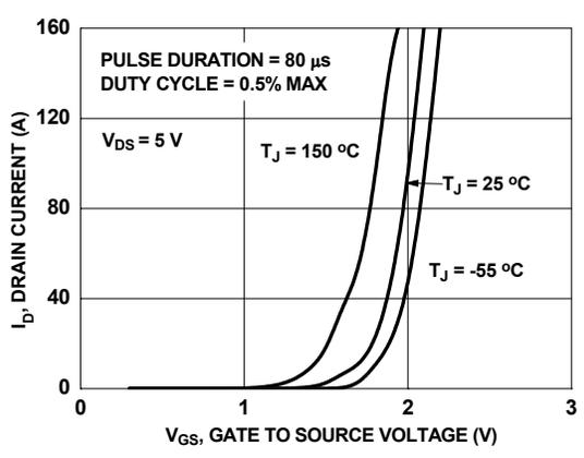
Figure 5. Transfer Characteristics
