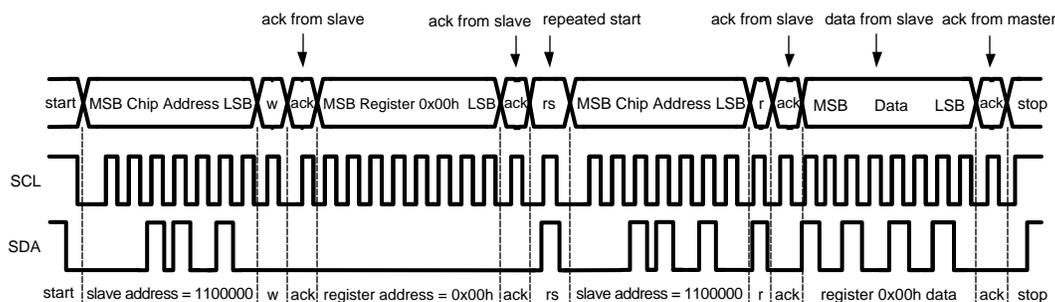
Figure 32. Example I<sup>2</sup>C Read Cycle
