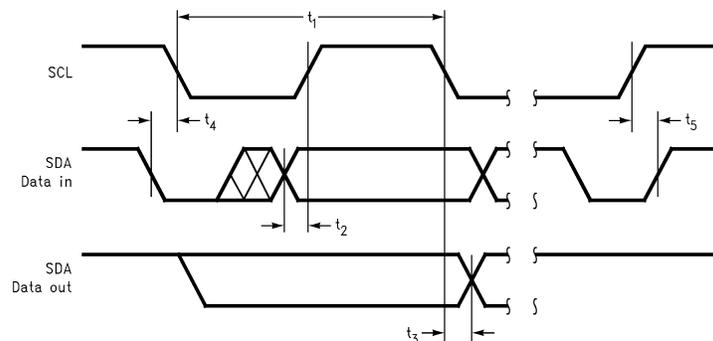
Figure 29. I<sup>2</sup>C Timing Diagram
