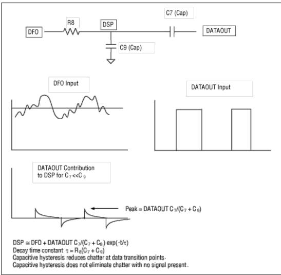
data filter, so that it does not make the filtered signal too sluggish.
