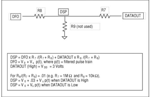
Figure 10. Resistive hysteresis circuit for squelch function.
