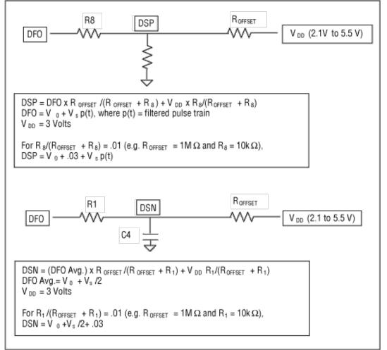
Figure 9. Two simple squelch circuits using a supply voltage.
