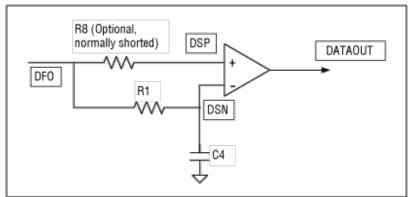
Figure 4. Fundamental data-slicing circuit.
