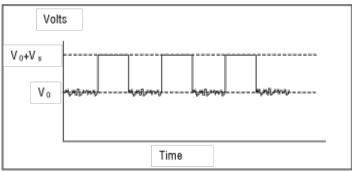
Figure 1. ASK demodulator output.
