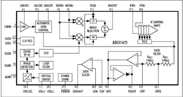
Figure 2. Block diagram of the MAX1473 ASK receiver.
