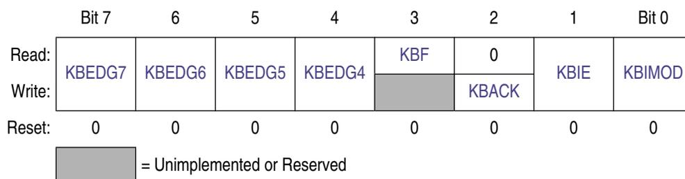
Figure 9-4. KBI Status and Control Register (KBI1SC)
