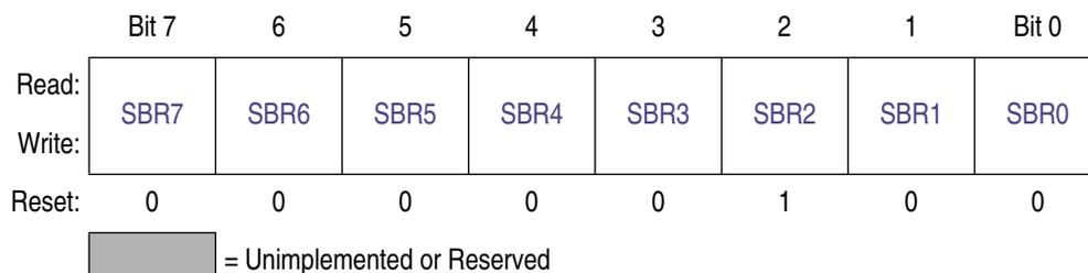
**Figure 11-6. SCI x Baud Rate Register (SCIxBDL)**
