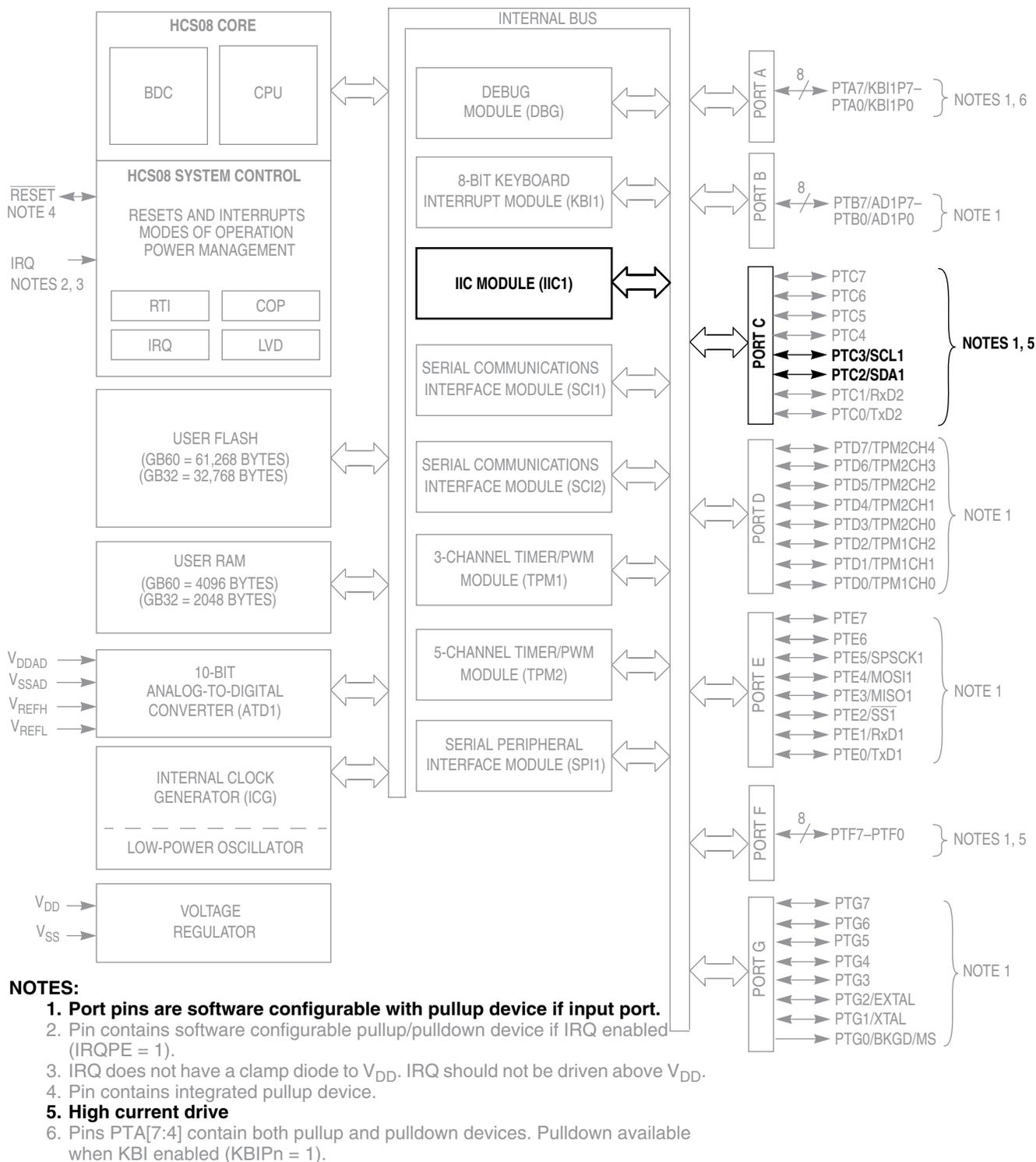
Figure 13-1. Block Diagram Highlighting the IIC Module
