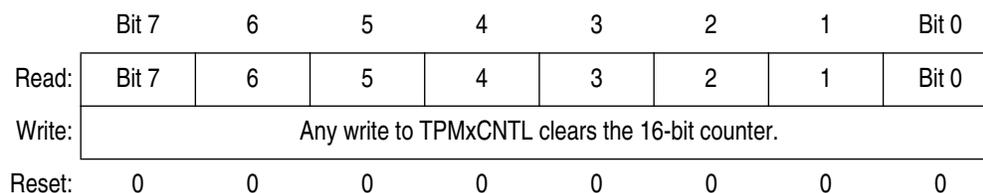
**Figure 10-7. Timer x Counter Register Low (TPMxCNTL)**
