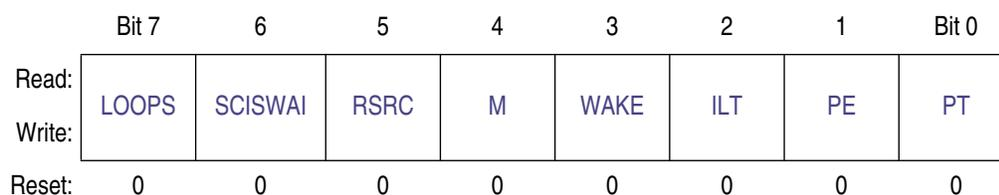
**Figure 11-7. SCI x Control Register 1 (SCIxC1)**
