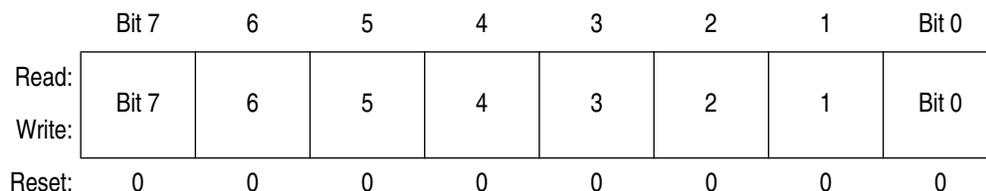
**Figure 10-12. Timer x Channel Value Register Low (TPMxCnVL)**
