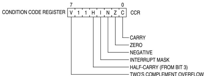
Figure 8-2. Condition Code Register
