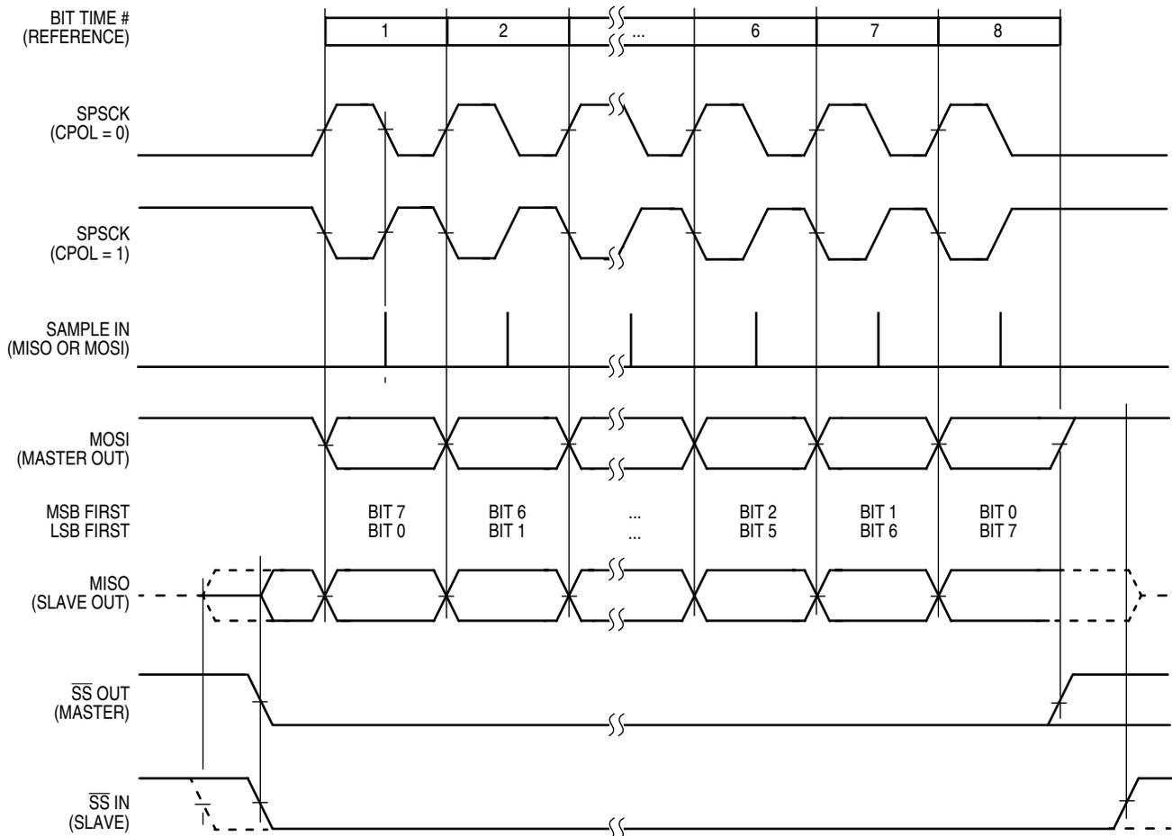
Figure 12-5. SPI Clock Formats (CPHA = 1)
