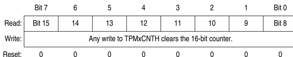
**Figure 10-6. Timer x Counter Register High (TPMxCNTH)**
