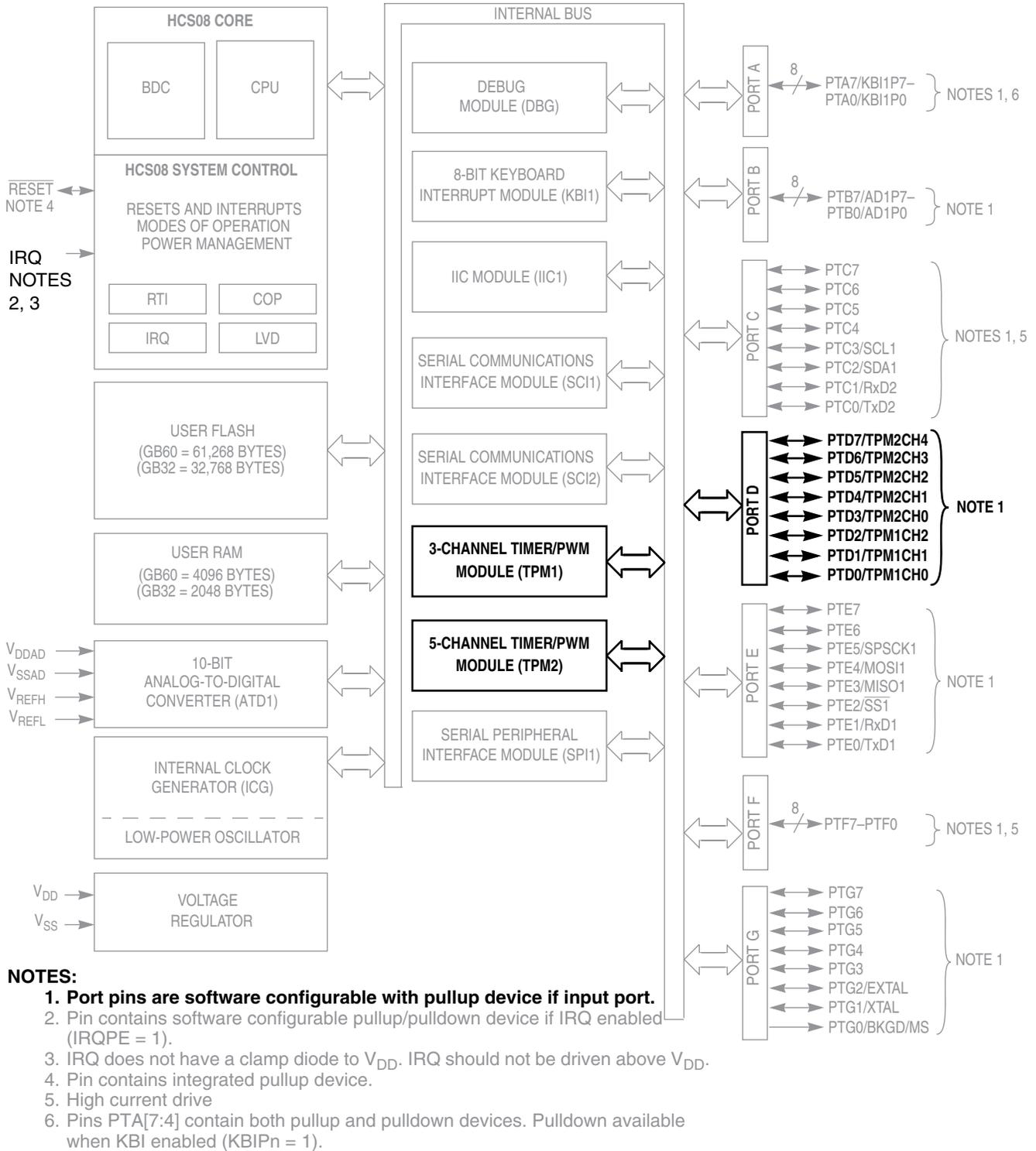
Figure 10-1. Block Diagram Highlighting the TPM Modules
