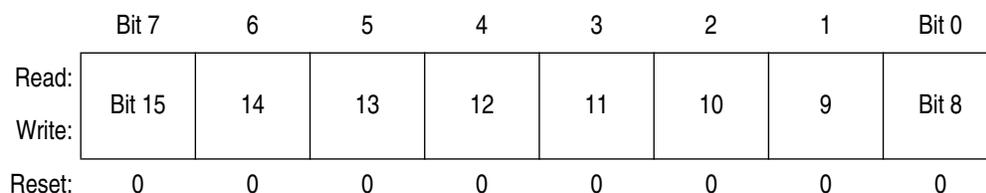
**Figure 10-11. Timer x Channel Value Register High (TPMxCnVH)**
