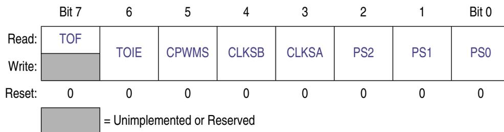
**Figure 10-5. Timer *x* Status and Control Register (TPM<sub>x</sub>SC)**
