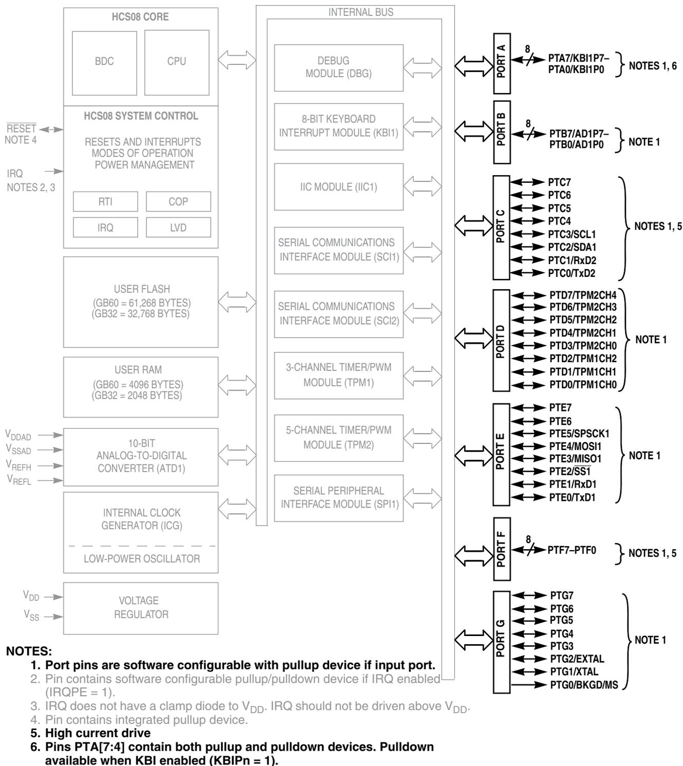
Figure 6-1. Block Diagram Highlighting Parallel Input/Output Pins
