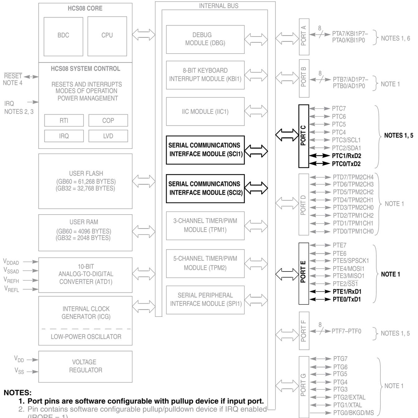
Figure 11-1. Block Diagram Highlighting the SCI Modules
