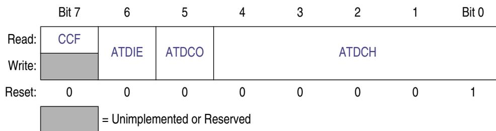
**Figure 14-8. ATD Status and Control Register (ATD1SC)**
