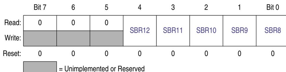
**Figure 11-5. SCI Baud Rate Register (SCIxBDH)**
