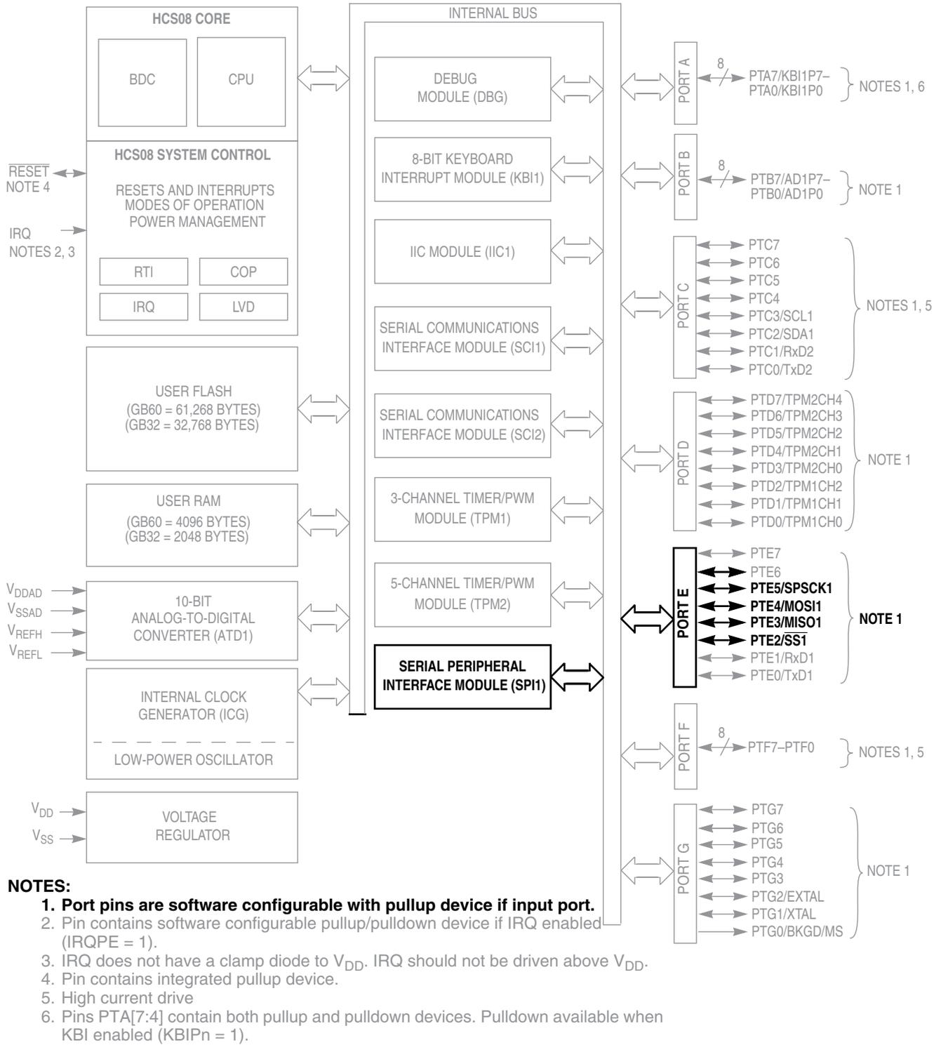
Figure 12-1. Block Diagram Highlighting the SPI Module
