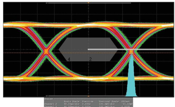
**Figure 3 - HDMI 1.4 Eye Pattern with RClamp0524PQ**
