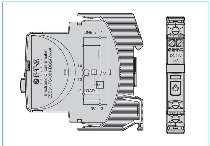
**ESS31-T Signal inputs / outputs (wiring diagrams)**
