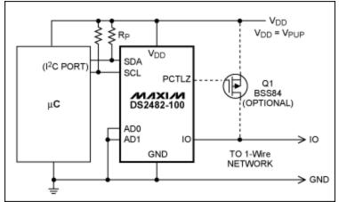
Figure 6. I<sup>2</sup>C interface with optional circuit for **extra strong** pullup (dashed lines).
