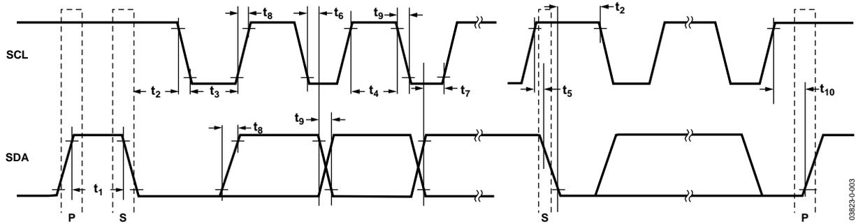
Figure 23. I<sup>2</sup>C Interface Timing Diagram
