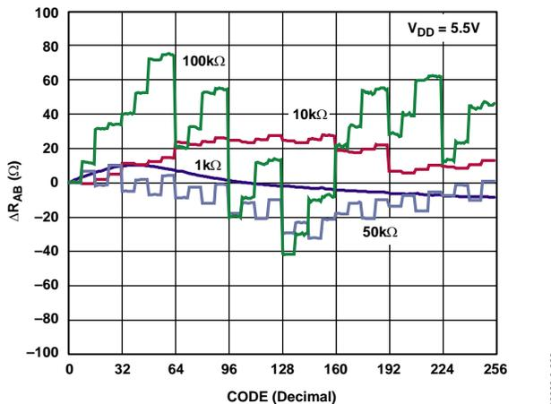
Figure 17. AD5252  $\Delta R_{AB}$  vs. Code,  $T_A = 25^\circ\text{C}$
