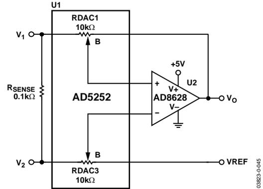
Figure 45. Current-Sensing Amplifier
