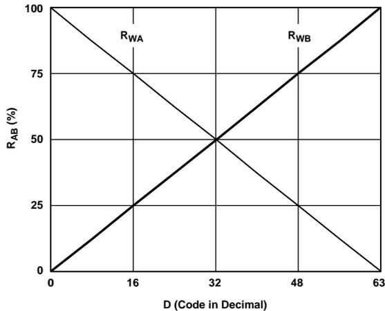
Figure 42. AD5251  $R_{WA}(D)$  and  $R_{WB}(D)$  vs. Decimal Code
