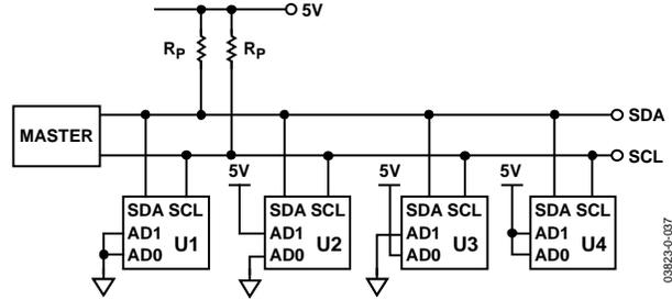
Figure 37. Multiple AD5251/AD5252 Devices on a Single Bus
