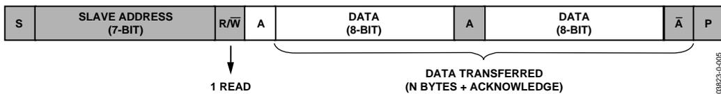
Figure 25. I<sup>2</sup>C—Master Reading Data from Slave
