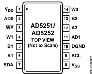
Figure 2. Pin Configuration
