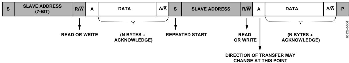
Figure 26. I<sup>2</sup>C—Combined Write/Read
