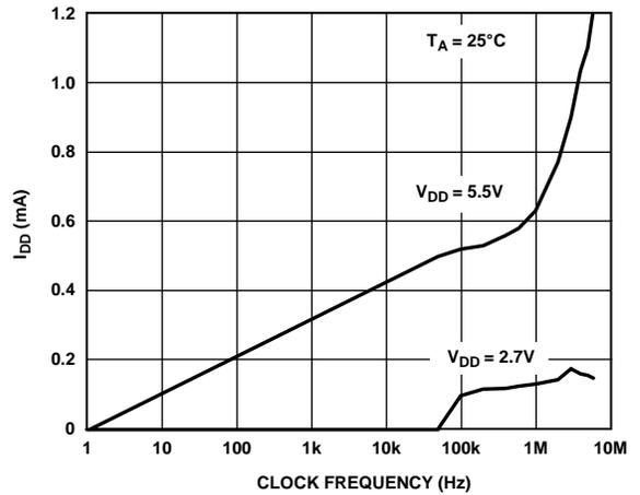
Figure 18. Supply Current vs. Digital Input Clock Frequency
