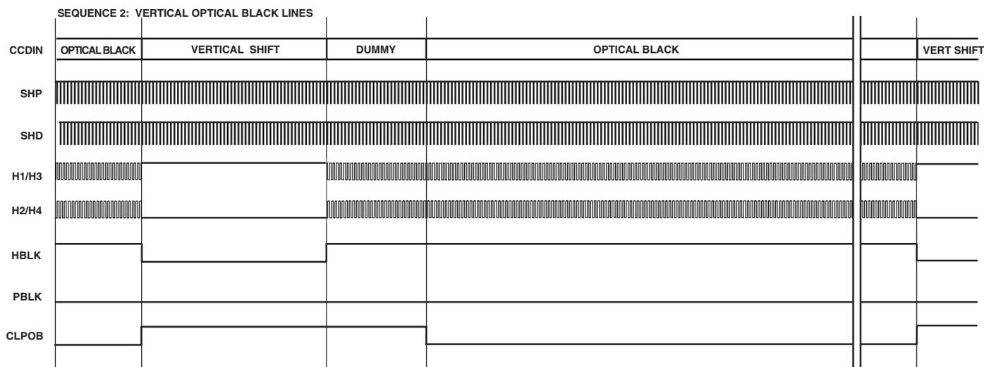
Figure 26. Horizontal Sequences during Vertical Optical Black Pixels
