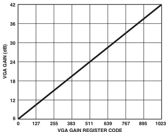
Figure 20. VGA Gain Curve (PxGA Not Included)
