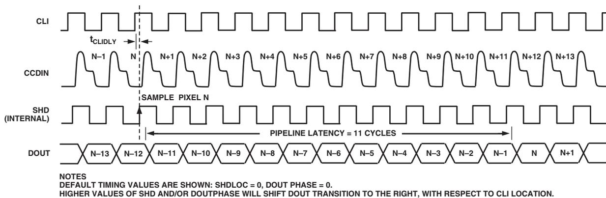
Figure 7b. Pipeline Delay for Digital Data Output
