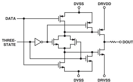
Circuit 3. Data Outputs D0-D9 (Pins 2-4, 7-13)
