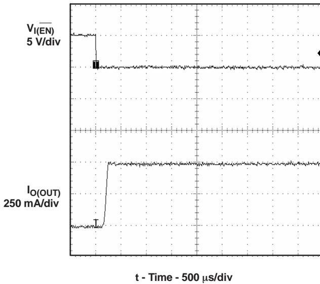
Figure 6. Short-Circuit Current, Device Enabled Into Short
