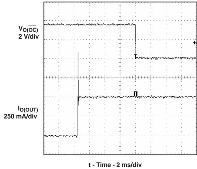
Figure 9. 3-Ω Load Connected to Enabled Device
