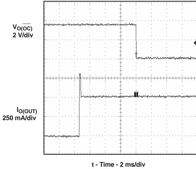
Figure 8. 4-Ω Load Connected to Enabled Device
