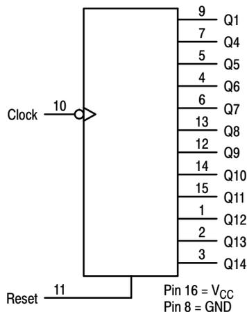
Figure 1. Logic Diagram
