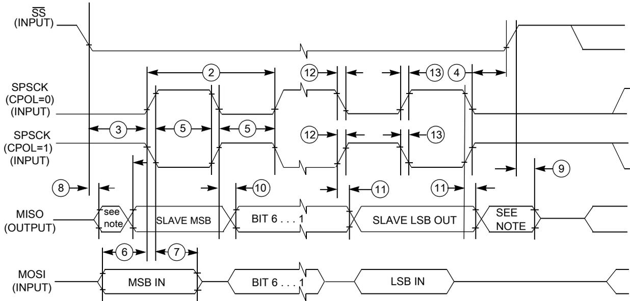
Figure 26. LPSPI slave mode timing (CPHA = 0)
