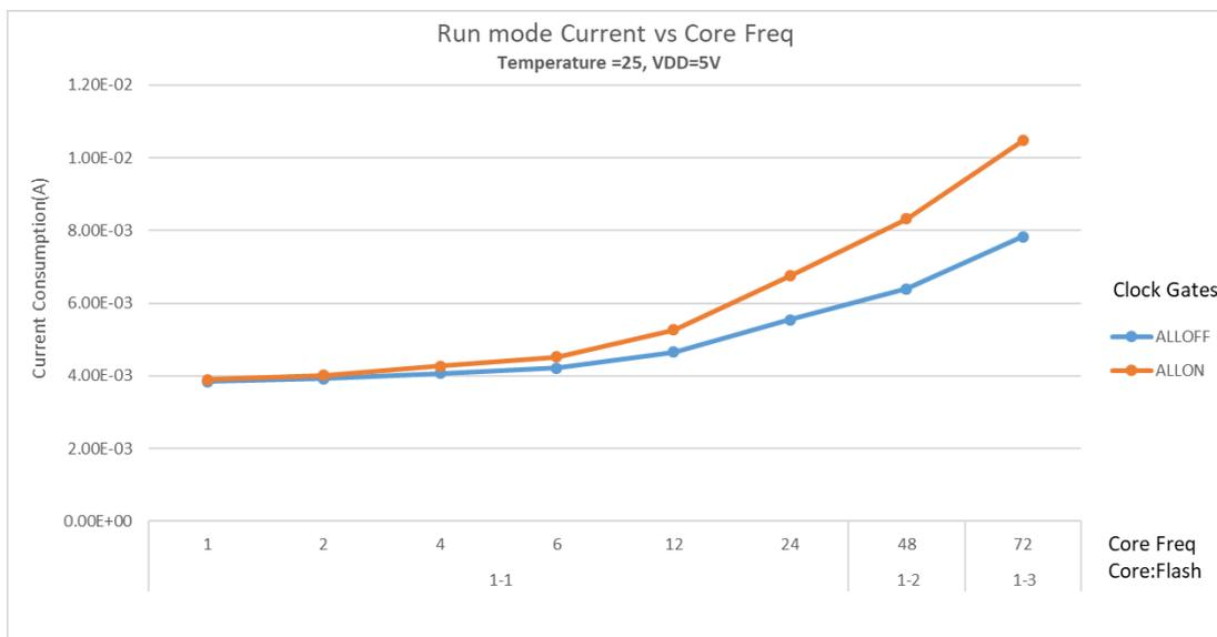
**Figure 15. Run mode supply current vs. core frequency**
