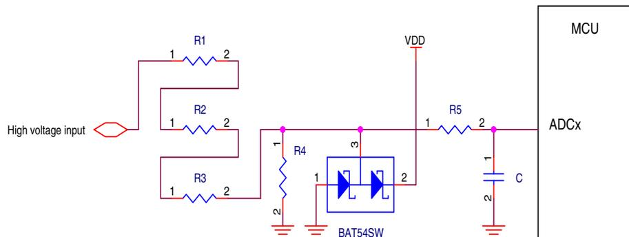
**Figure 31. High voltage measurement with an ADC input**
