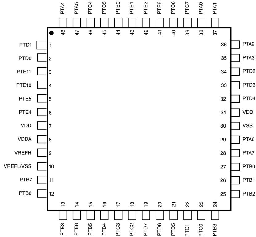
Figure 7. 48 LQFP Pinout Diagram
