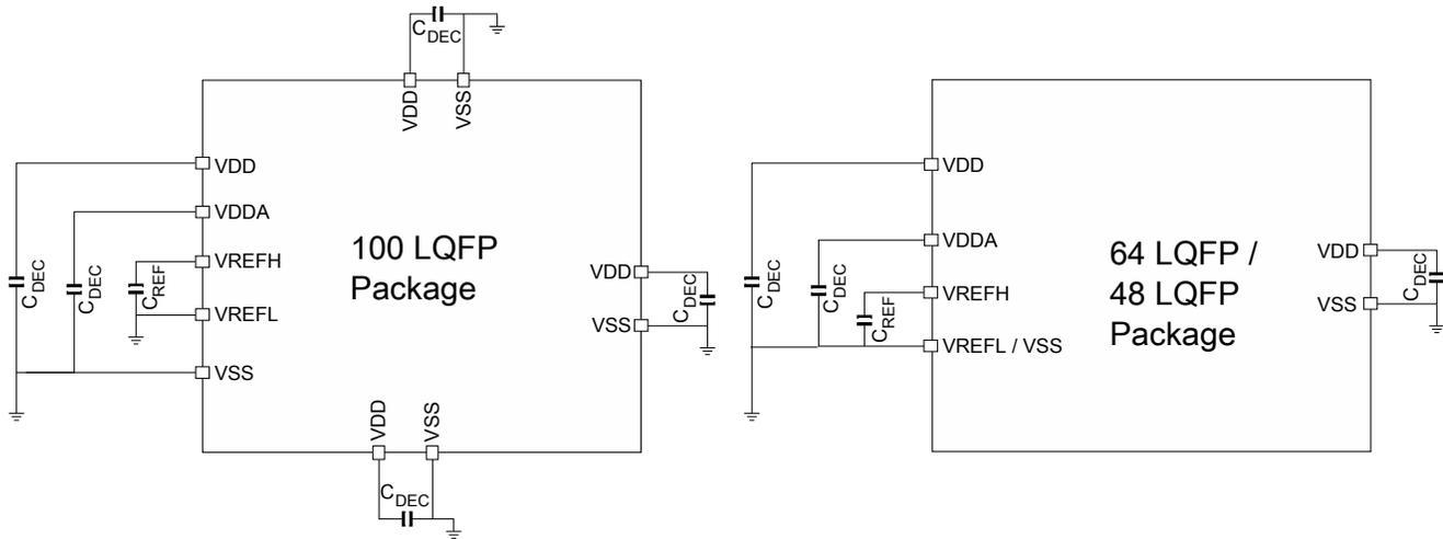
Figure 14. Pinout decoupling
