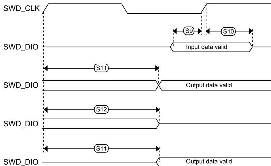
**Figure 29. Serial wire data timing**
