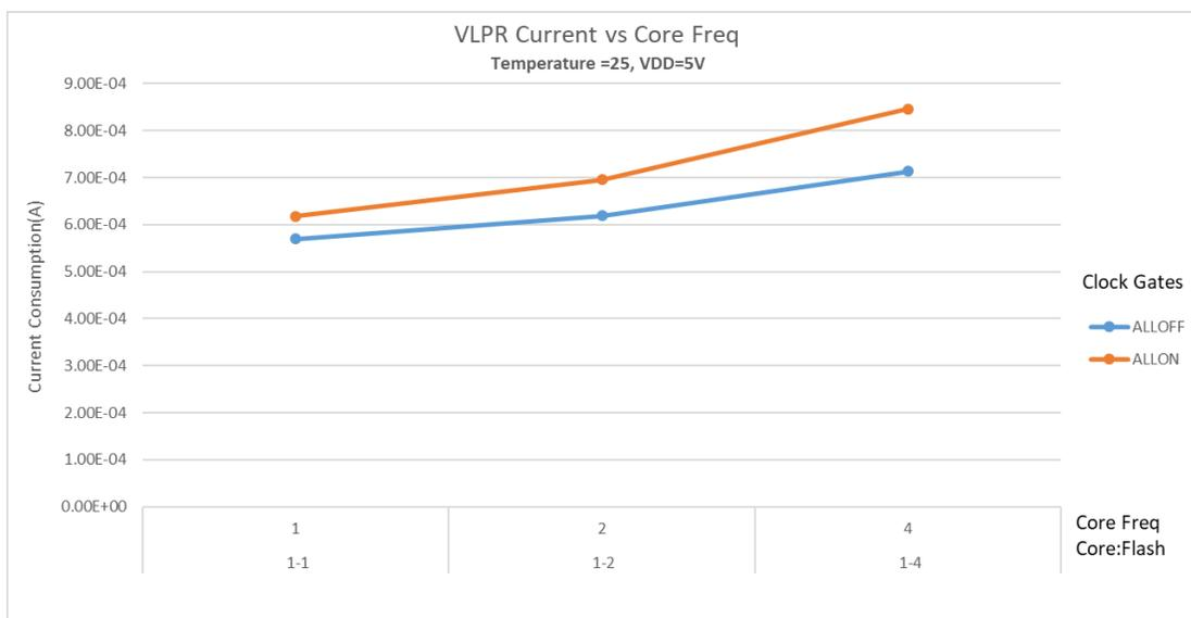
**Figure 16. VLPR mode supply current vs. core frequency**
