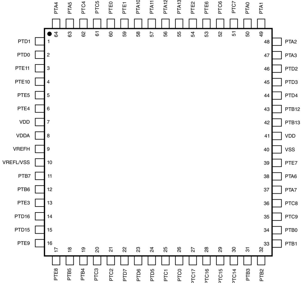
**Figure 6. 64 LQFP Pinout Diagram**
