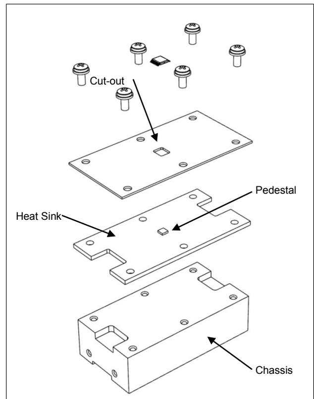
12. Due to the high power dissipation of this part, a heat sink must be attached to the printed circuit board.
