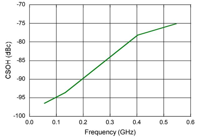
**Typical Distortion Performance Curves: 79 NTSC + 75 ATSC  $V_0 = +44$  dBmV Flat @ +25°C**
