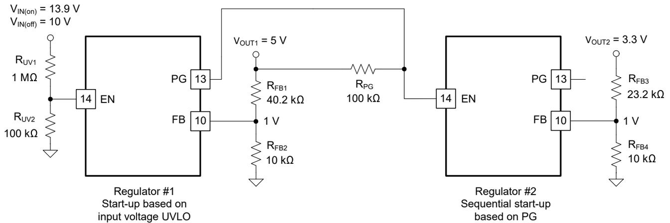
**Figure 7-4. TLVM13630 Sequencing Implementation Using PG and EN**
