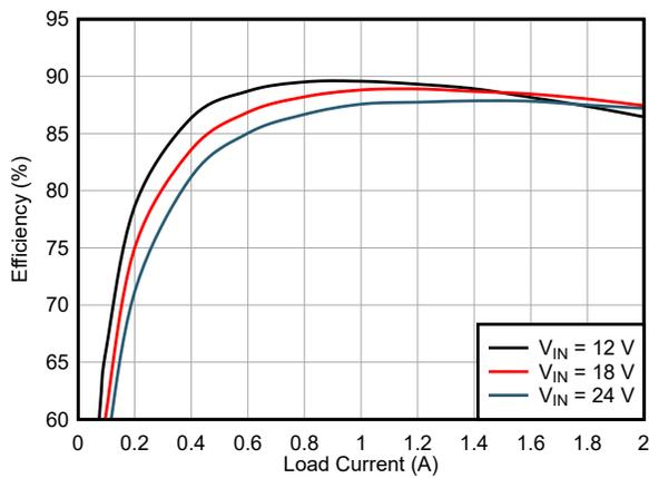
**Figure 8-13. Efficiency Curves**
