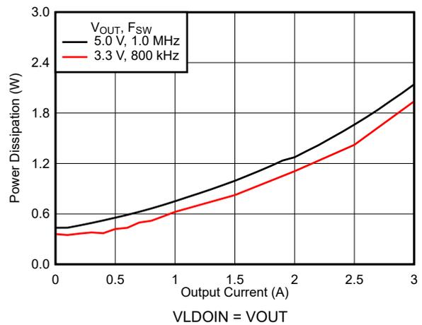
Figure 6-19. Power Dissipation
