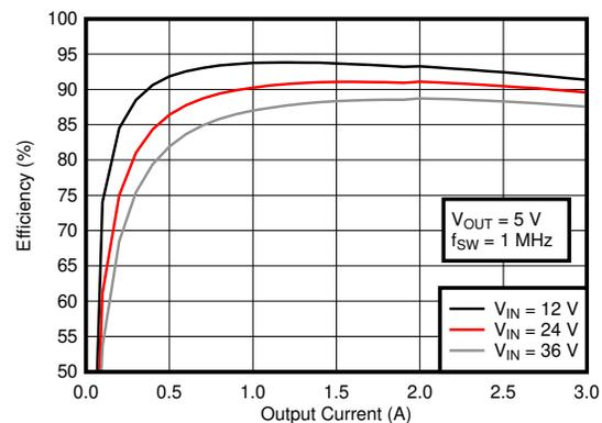
Typical Efficiency, V<sub>OUT</sub> = 5 V, F<sub>SW</sub> = 1 MHz
