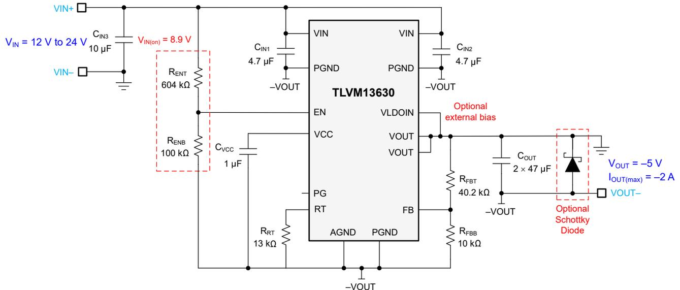
Figure 8-12. Circuit Schematic
