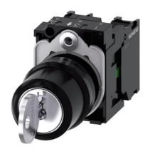
RONIS key-operated switch, 22 mm, round, plastic, lock number SB30, with 2 keys, 3 switch positions I-O-II, latching, 10:30h/12h/13:30h, Key removal I+O+II, with holder, 1 NO, 1 NO, screw terminal, possible special locks: SB31, 421, 455, with laser labeling, upper case and lower case, always upper case at the beginning of the word
