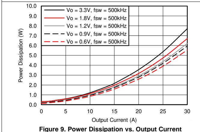
Figure 9. Power Dissipation vs. Output Current
