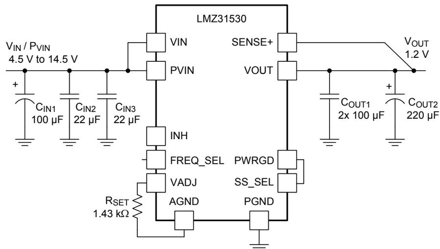
**Figure 17. Typical Schematic**
