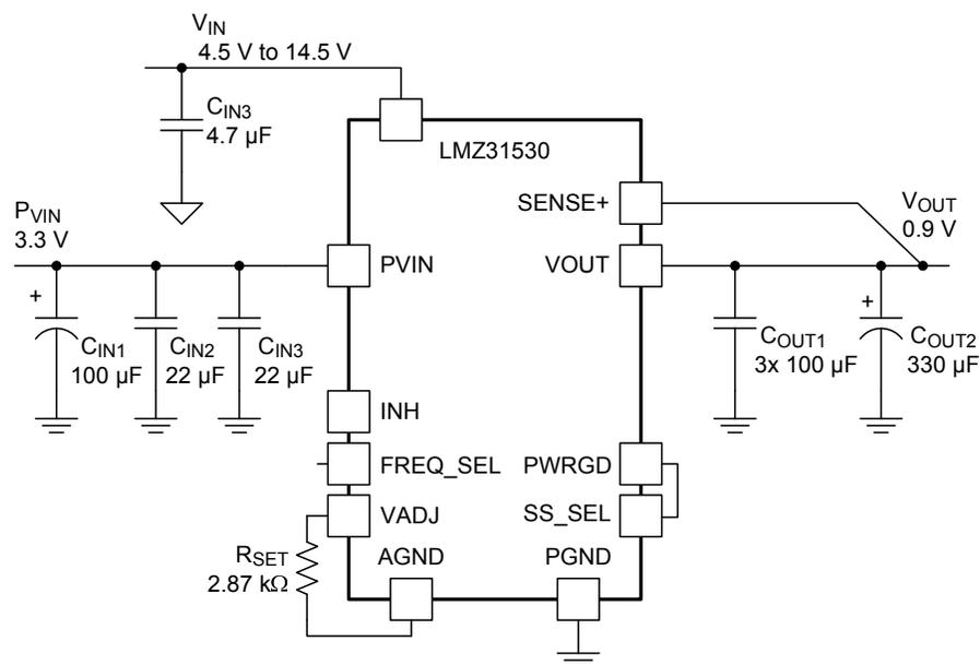
**Figure 18. Typical Schematic**
