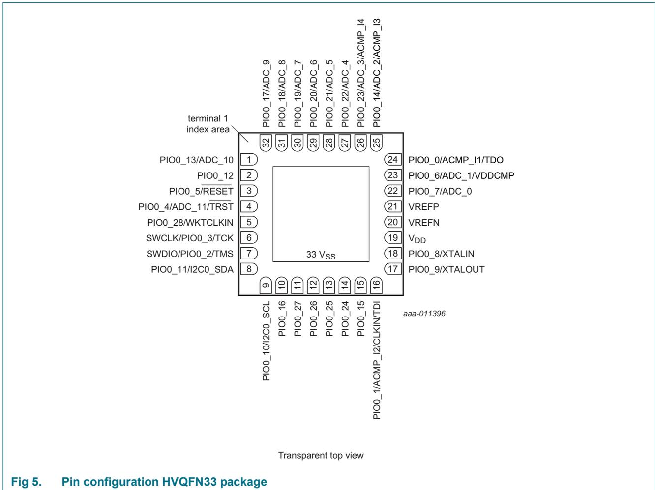
Fig 5. Pin configuration HVQFN33 package
