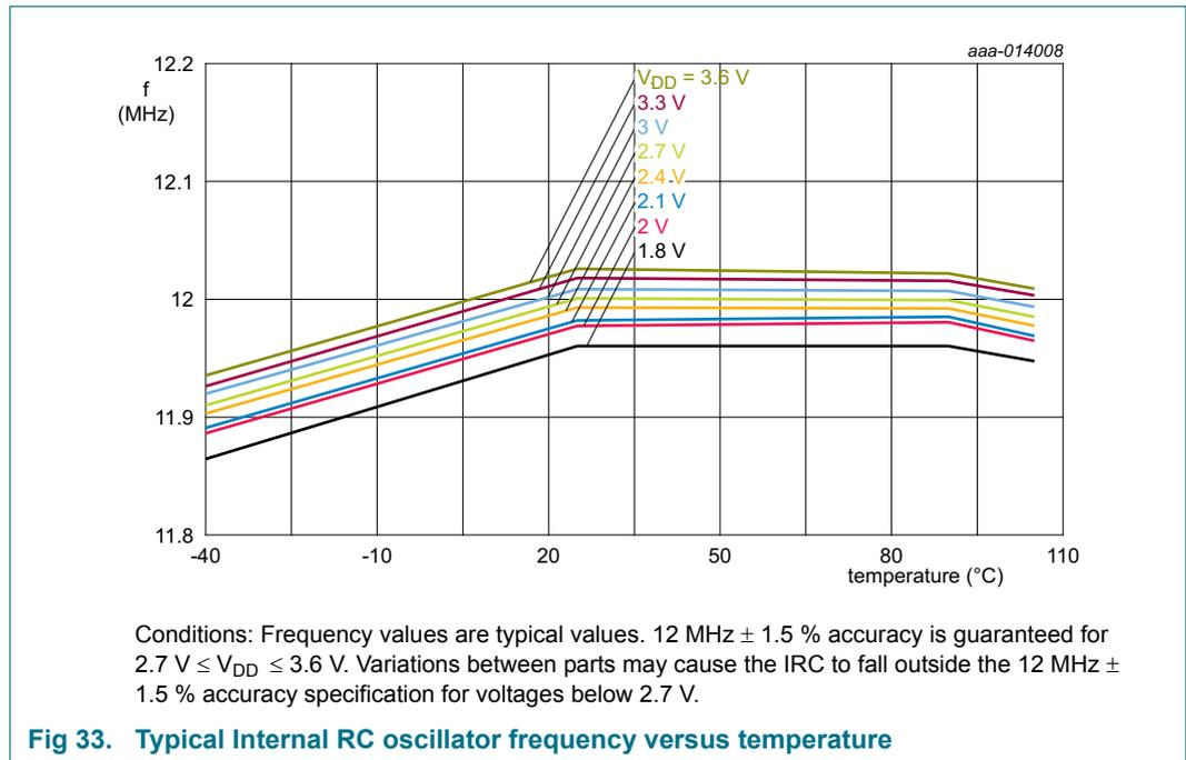
**Fig 33. Typical Internal RC oscillator frequency versus temperature**
