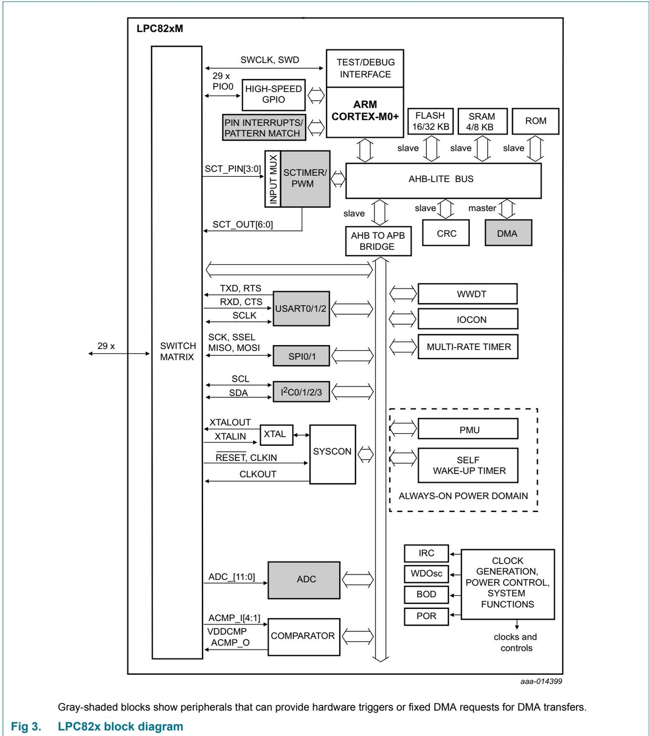
Gray-shaded blocks show peripherals that can provide hardware triggers or fixed DMA requests for DMA transfers.
