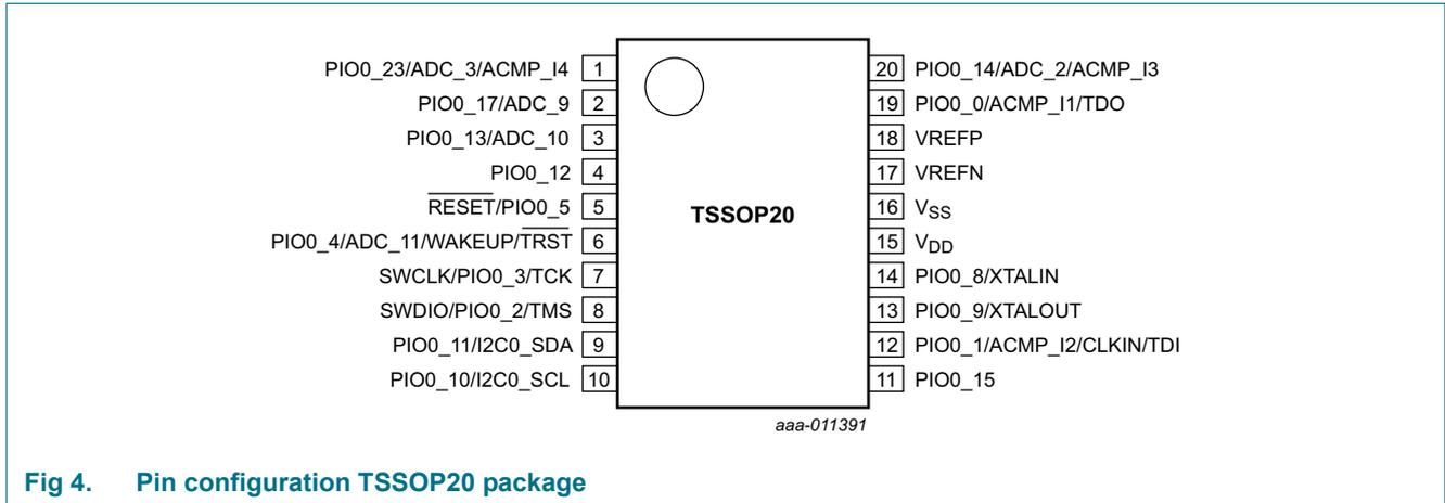
Fig 4. Pin configuration TSSOP20 package
