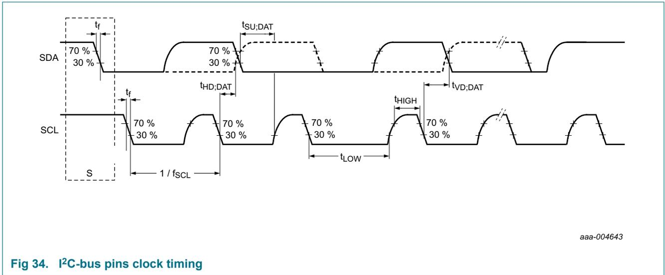
Fig 34. I<sup>2</sup>C-bus pins clock timing
