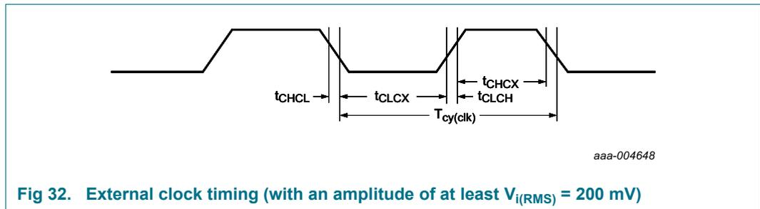
**Fig 32. External clock timing (with an amplitude of at least  $V_{i(RMS)} = 200\text{ mV}$ )**
