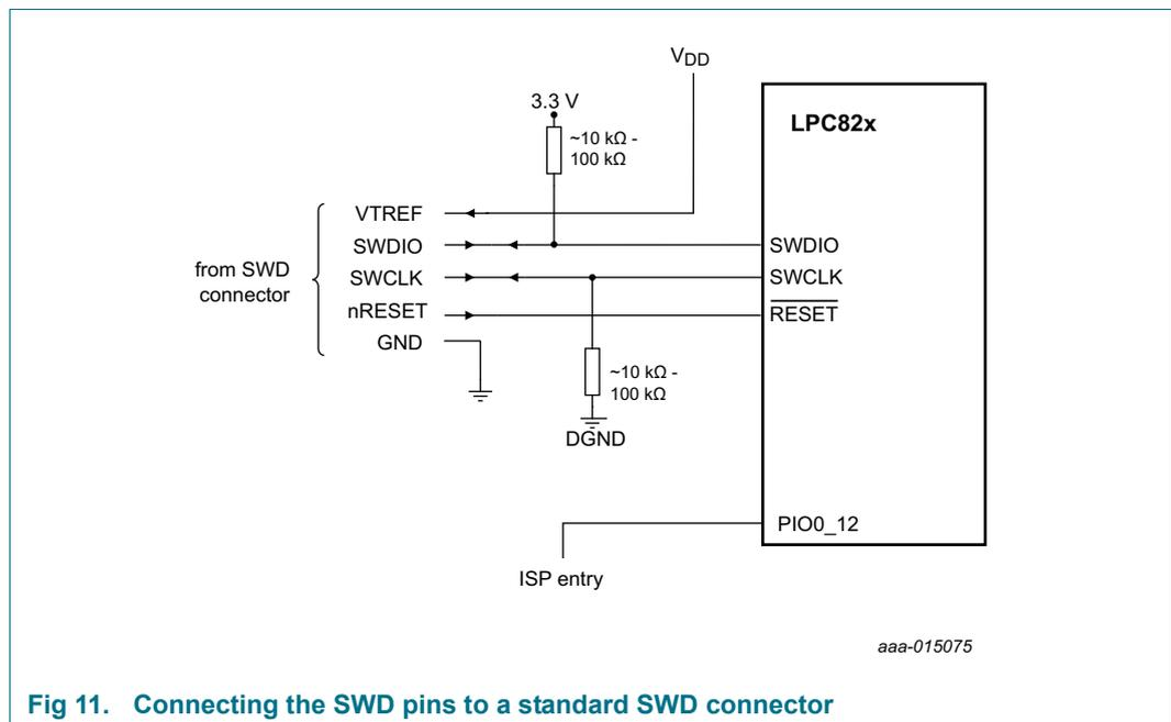
**Fig 11. Connecting the SWD pins to a standard SWD connector**
