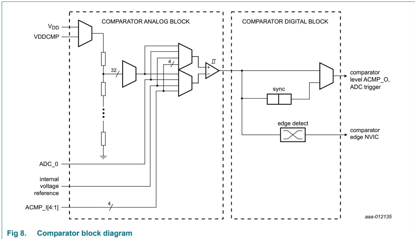
Fig 8. Comparator block diagram
