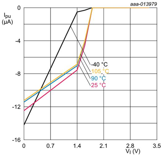
Conditions:  $V_{DD} = 1.8$  V; standard port pins.
