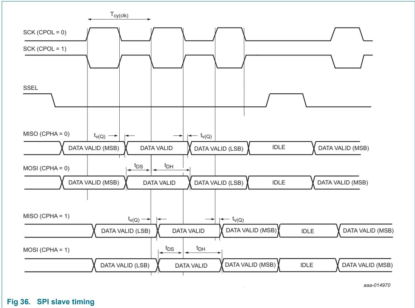
Fig 36. SPI slave timing
