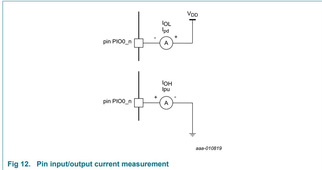
**Fig 12. Pin input/output current measurement**
