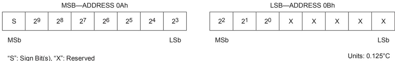
**Note:** Temperature and battery voltage (V<sub>IN</sub>) are measured using the same ADC. Therefore, measurements are a 220ms average updated every 440ms.
