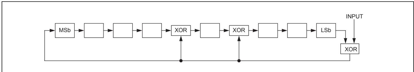
Figure 8. 1-Wire CRC Generation Block Diagram
